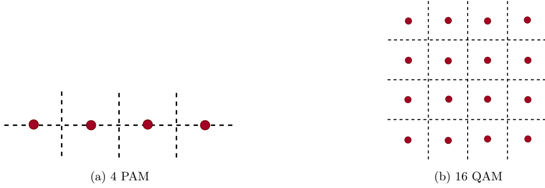
Figure 2.19: The decision regions of PAM for the AWGN channel and the ML rule.
