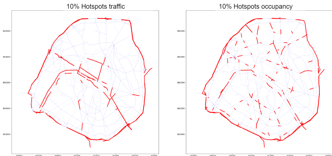
Figure II.2: Hotspots for traffic and congestion in Paris during a morning commute in 2014. Positions along the axes are given in meters in the Lambert 93 conformal conic projection system (EPSG:2154)
