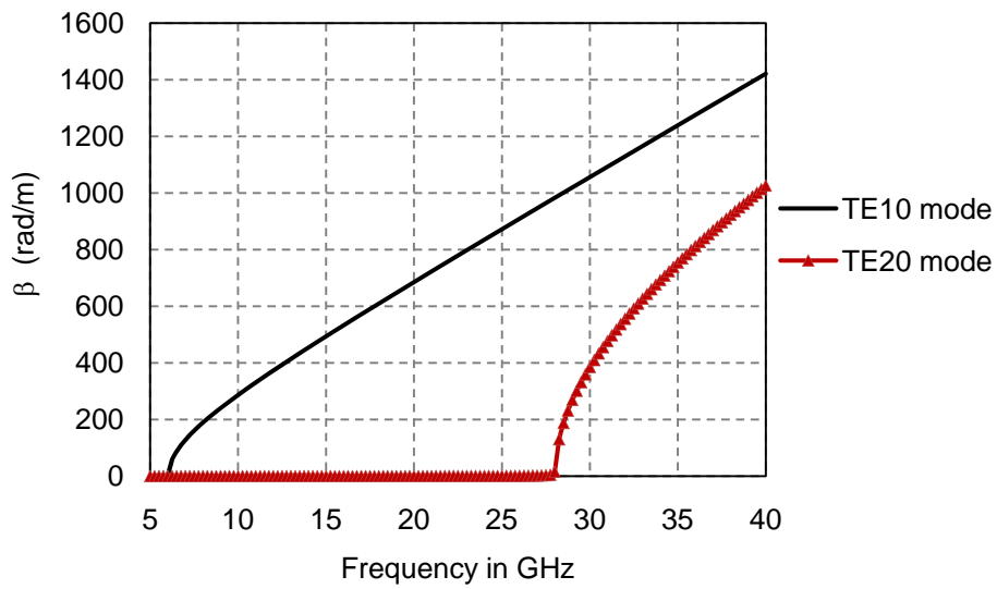
Fig. 3.13 Phase constants of the ridged waveguide illustrating the cutoff frequencies of the TE 10 and the TE 20 modes.
