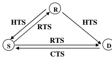
Figure 3.1.3.2: The exchange of control packets for CoopMAC.
