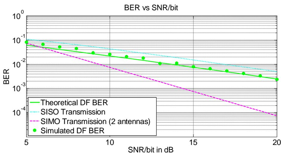
Figure 2.1.3: The performance of the DF transmission scheme.
