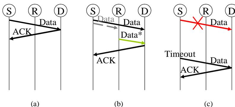
Figure 5.1.5: Message flows of (a) Non-cooperative transmissions (b) Cooperative transmissions and (c) Non-cooperative transmissions with re-transmission processes
