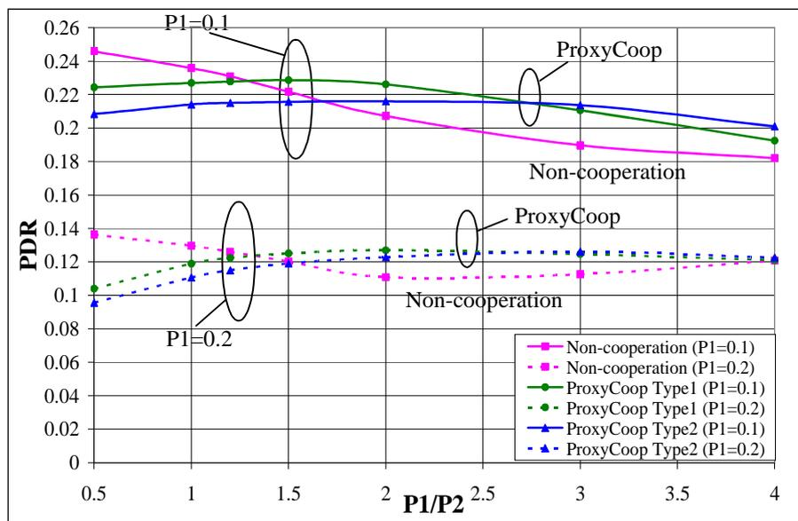
Figure 5.4.3.10: PDR of non-cooperative and ProxyCoop transmissions in the 8-terminal network.
