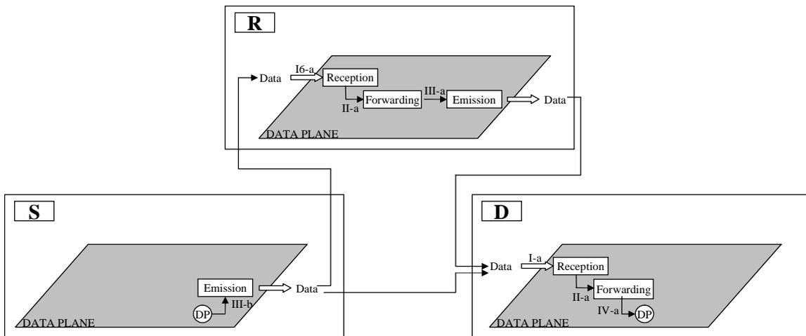
Figure 4.2.1: A data transmission method in cooperative communications.
