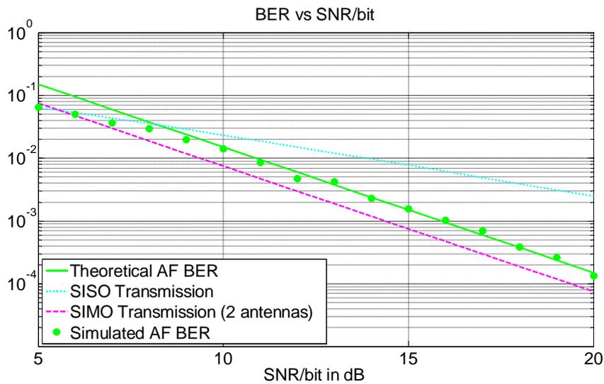
Figure 2.1.2: The performance of the AF transmission scheme.
