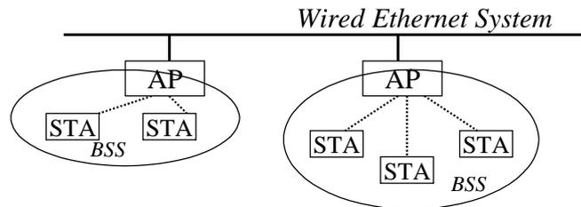
Figure 6.3.1: Network architecture of IEEE 802.11 WLANs.
