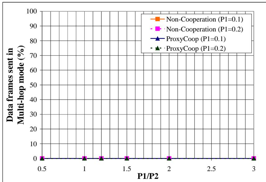
Figure 5.4.3.1: The percentage of data frames sent in multi-hop mode in scenario 1.
