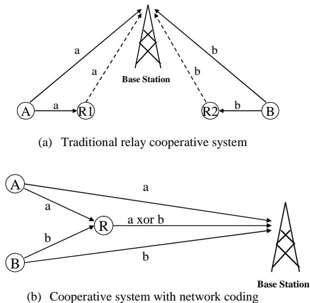
Figure 2.4.2: (a) Traditional relay cooperative system and (b) Cooperative system with network coding in a cellular network.
