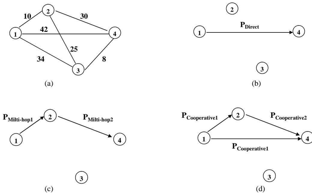
Figure 3.2.1.1: An illustrative network with link costs in term of minimum power requirement for data transmissions.
