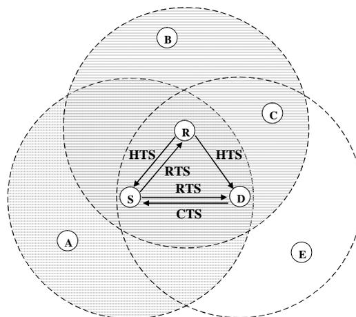
Figure 3.1.3.4: Hidden terminal problems in CoopMAC method.
