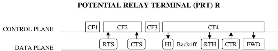
Figure 4.4.2.2: Data plane and control plane interactions of the DCM protocol at a PRT R.
