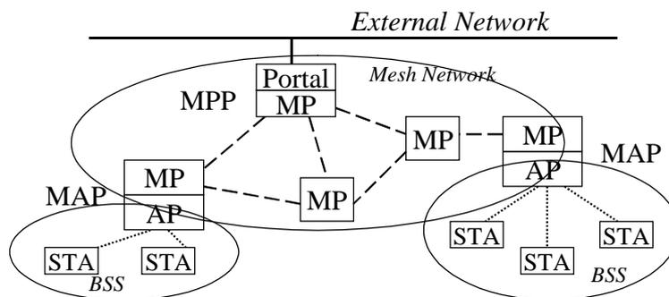
Figure 6.3.2: Network architecture of IEEE 802.11s WMNs.
