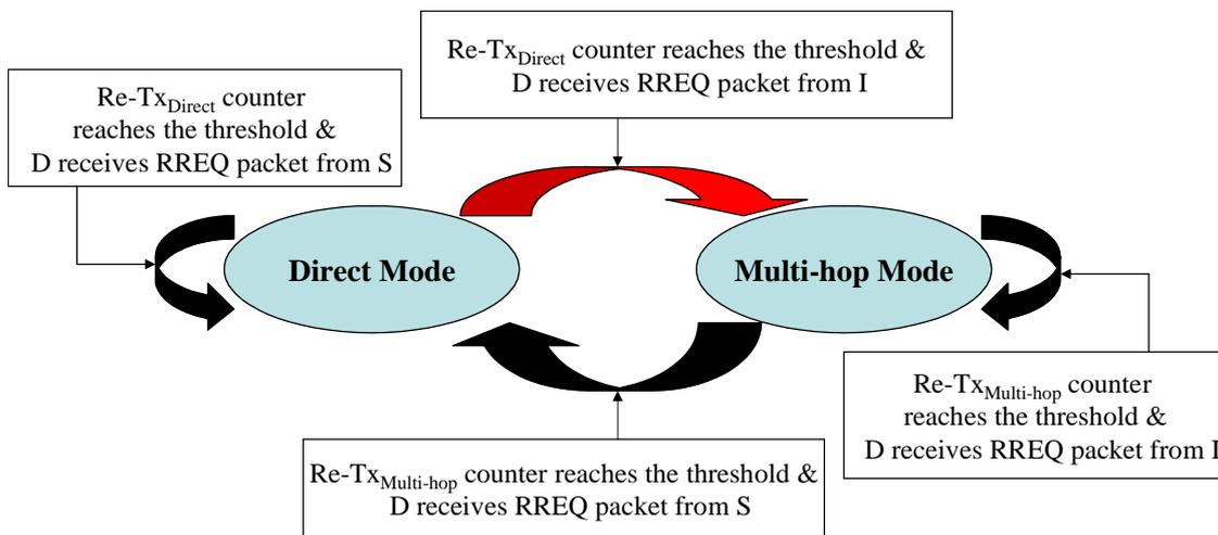
Figure 5.1.4: Transmission mode transition of non-cooperative transmission.
