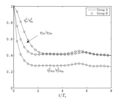
FIGURE 5.8: The evolution of statistics of the two groups of particles, A, B, in the same fluid realization, in time after the two-way coupling is turned on, group A is active and B is ghost particles.
