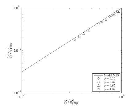
FIGURE 5.12: Relation 5.96 to calculate the mesoscopic particle energy.
