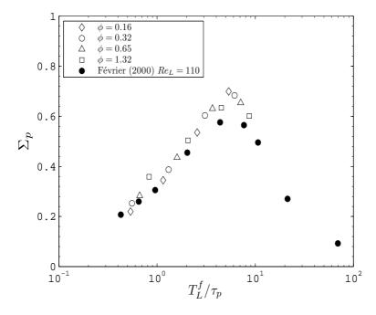
Figure 7.18: Preferential concentration measured in two-way coupled flows.
