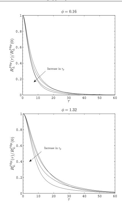
Figure 7.4: Modification of the Lagrangian correlations of fluid velocity correlation viewed by the particles for lowest and highest mass loadings
