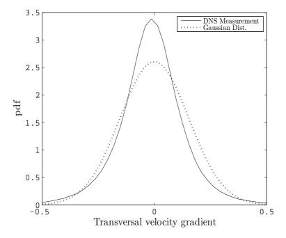
Figure 2.12: Probability distribution of the transversal derivative of velocity fluctuations of the flow field obtained using stochastic forcing.
