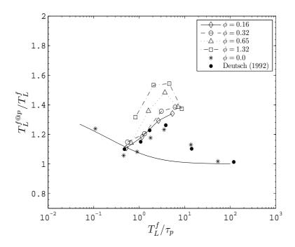
FIGURE 7.15: Modification of the Lagrangian timescale  $T_L^{f@p}$  viewed by the particles due to the particles,  $T_L^f$  corresponds to the Lagrangian timescale of the two-way coupled flow, solid line is the relation 7.22 for the  $T_L^f/T_E = 0.727$  (mean value over the ensemble of simulations)
