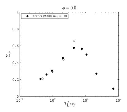
Figure 7.17: Preferential concentration measured in one-way coupled flows.
