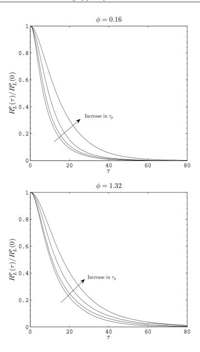
Figure 7.2: Modification of the Lagrangian correlations of particle fluctuation velocity for lowest and highest mass loadings.
