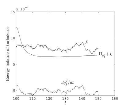
FIGURE 6.3: Turbulent kinetic energy balance in presence of particles (Simulation  $\phi = 0.16$  and  $St_0 = 2.0, Re_L = 96$ )
