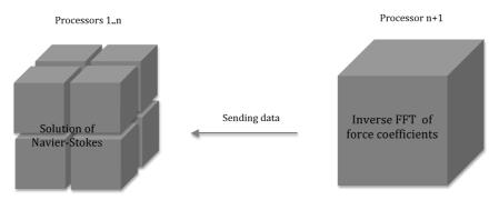
FIGURE 2.3: Representative figure showing the configuration of simulations to perform inverse FFT in parallel platform.
