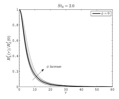
Figure 6.18: Modification of the Lagrangian one-point correlations, for large inertia particles
