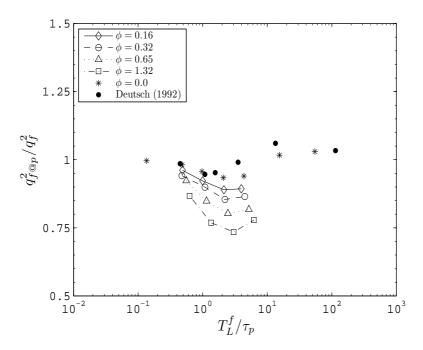
FIGURE 7.14: Modification of the fluid kinetic energy  $q_{f@p}^2$  viewed by the particles due to the particles,  $q_f^2$  corresponds to the fluid kinetic energy of the two-way coupled flow.
