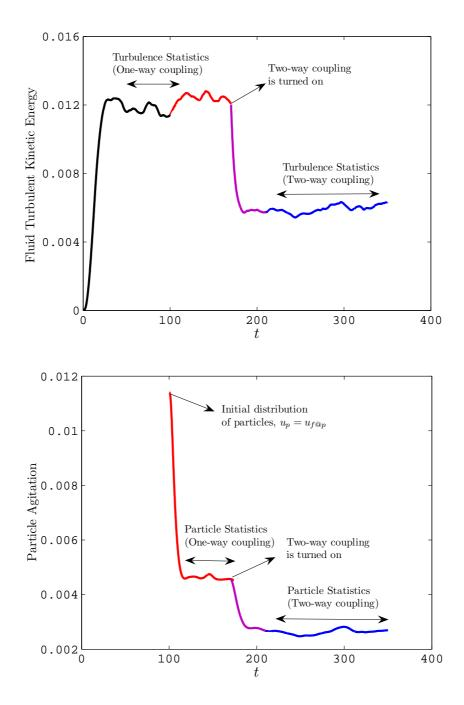
FIGURE 6.2: Representative figures showing the making of statistics for one-way and two-way coupled flows, for particles and turbulence
