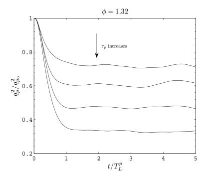
Figure 7.1: Behaviour of particle agitation,  $q_p^2$ , with the particle inertia  $\tau_p$  (see the relation 7.8)
