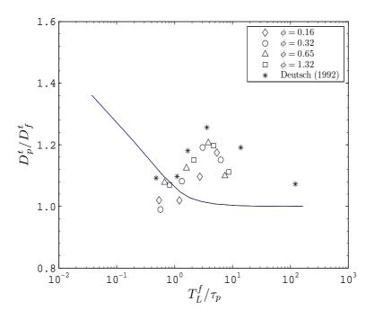
Figure 7.12: Modification of the dispersion coefficient with reference to the diffusion coefficient of fluid elements due to the two-way coupling, solid line corresponds to the theory of Pismen and Nir (1978).
