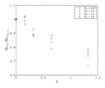
FIGURE 6.7: Modification of the turbulent Reynolds number,  $Re_L$
