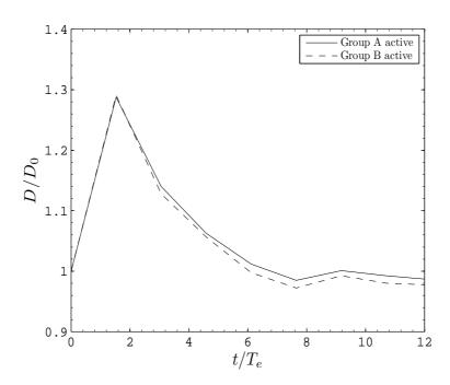
FIGURE 5.11: Statistical difference between the particle source terms  $f_{u_i}$  of the two groups A, B introduced into the same fluid realization; solid line: group A is active, B is ghost, dashed line: group B is active, A is ghost.
