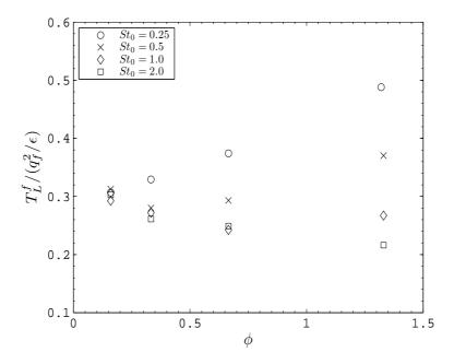
FIGURE 6.20: Ratio of the Lagrangian timescale  $T_L^f$  to the characteristic turbulence timescale  $q_f^2/\epsilon$ , see relation 6.17
