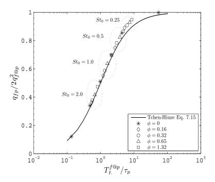
Figure 7.6: Then-Hinze relation 7.15 verified for two-way coupled flows compared to the one-way coupled flows,  $\phi = 0$
