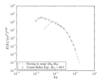
Figure 2.7: 3D kinetic energy spectrum of the flow field obtained using stochastic forcing. characterized by the Gaussian distribution.
