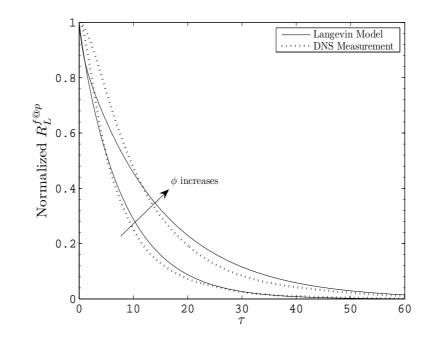
Figure 5.13: Comparison of the Langevin model 5.104 for the correlation of the fluid velocity viewed by the particles to the DNS measurements,  $St_0 = 0.25$
