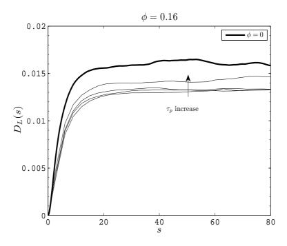
FIGURE 6.21: Modification of the Lagrangian structure function, for low mass loading
