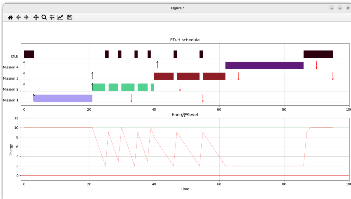
(b) Mission schedule using ED-H and precedence constraints. Both the dependent jobs and independent jobs release and deadline are marked as dashed arrows and continuous arrows.
