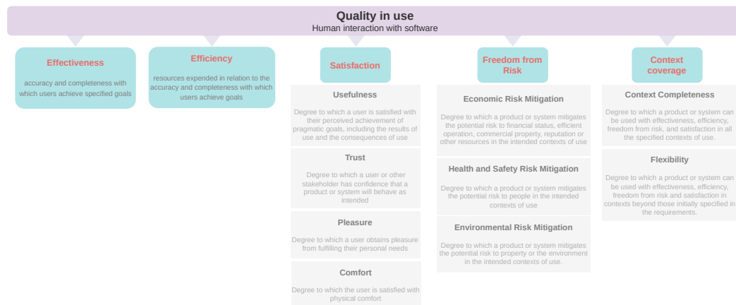
Figure A.2 Quality in use model proposed by the ISO 25010. It evaluates the quality characteristics of the software when it is used under specific context.
