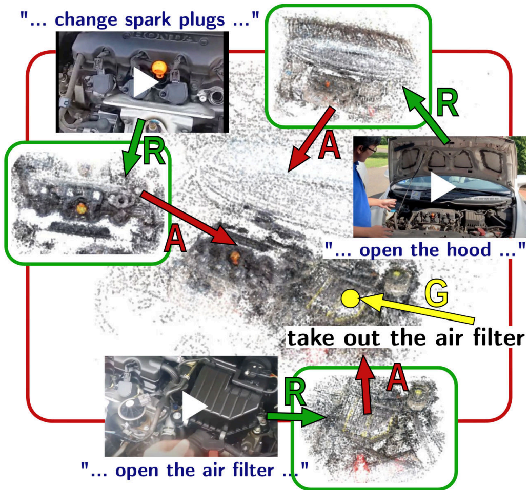
Figure 5.1: Illustration of the proposed method. Given a set of instructional videos showing the same object (e.g. same car model), we propose a two-step 3D reconstruction approach where, first, each video is independently reconstructed (R) and, second, reconstructions are aligned (A) in a single model. Using the reconstructed 3D model together with the narrations from each individual video and no manual supervision, we learn a language grounding model (G) that can determine the corresponding 3D region for a given text query such as “air filter”.
