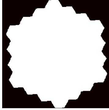
Figure 5.13: GTCAO test bench M1 pupil. It has no central obscuration (and no spider), and the orientation corresponds to a spin of 3.6 degrees.
