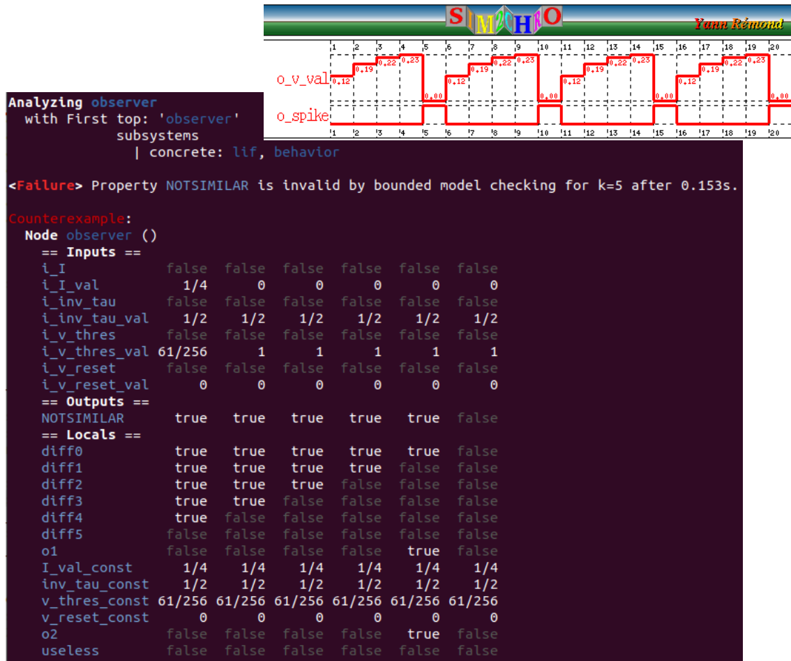
Figure 4.17: Results of Kind2 parameters exploration with the LIF neuron model, considering \Delta t_5 . Assertions were added on i\_inv\_tau and i\_v\_reset : 0.0 < i\_inv\_tau < 1.0 and i\_v\_reset = 0.0 . On top right, the simulation of the neuron LIF with the counterexample set of parameters.
