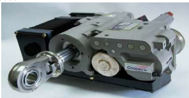
figure I-7 : Concept COVAN 13hp EHA Demonstrator
