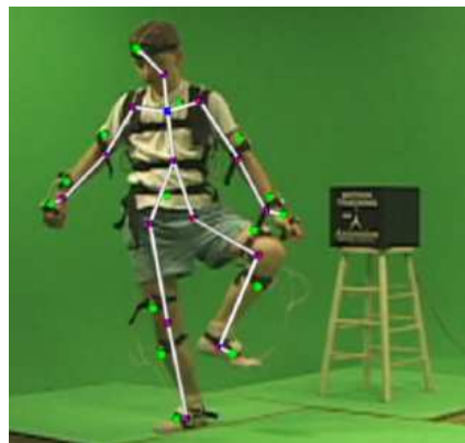
Figure 3.2: Human motion representation by joint centers: adapted from [O'Brien et al. 2000], the motion capture system used in this case was based on magnetic devices.
