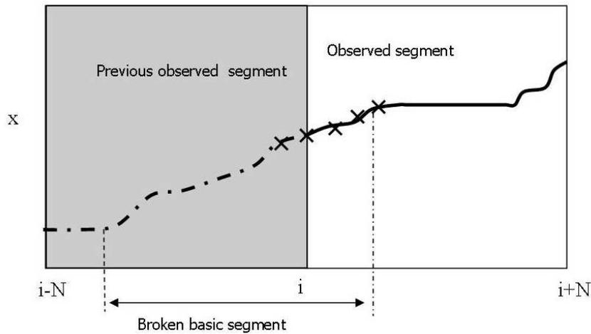
Figure 5.10: Planning the  $x$  component of the horizontal trajectory. To plan this trajectory we use the information of the basic segment. The via points are represented by cross marks, the observed segment (solid line) is in the white region, while the next segment is in the gray region( dashed line).
