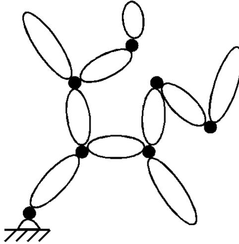
Figure 2.8: A robot manipulator with multiple kinematic chains.
