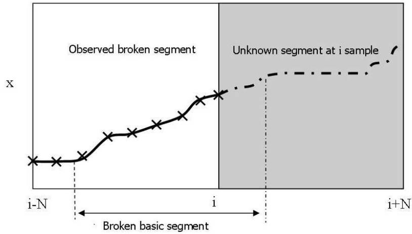
Figure 5.8: Planning the  $x$  component of the horizontal trajectory. The via points are represented by cross marks, the observed segment (solid line) is in the white region, while the next segment is in the gray region (dashed line).
