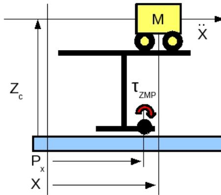
Figure 5.5: Cart-table model, represents the relationship between the ZMP,  $p$ , and the CoM,  $x$ , positions.  $\tau$  is the torque at  $p$  and  $M$  is the robot mass.
