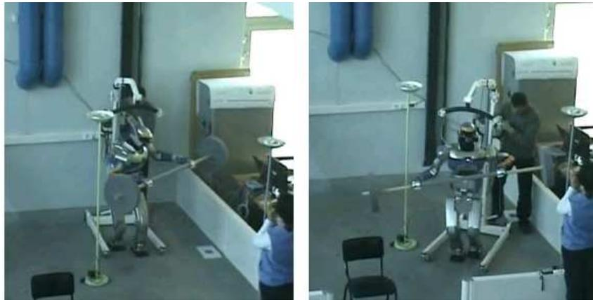
Figure 1.7: From [Esteves Jaramillo 2007]: the robot HRP-2 is carrying an object from one place to another while avoiding collisions between its own body, the manipulated object and the other objects in the environment.
