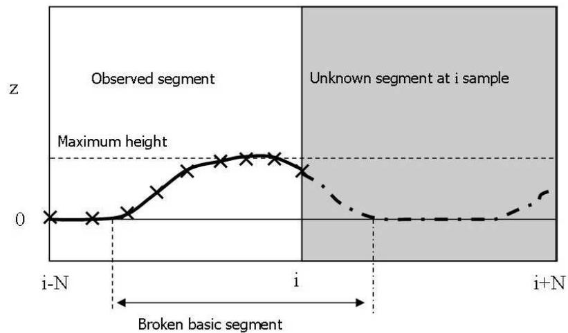
Figure 5.9: Planning the height  $Z$  trajectory. The via points are represented by cross marks, the observed segment (solid line) is in the white region, while the next segment is in the gray region (dashed line). The thin-horizontal-dashed line indicates the maximum allowed height.
