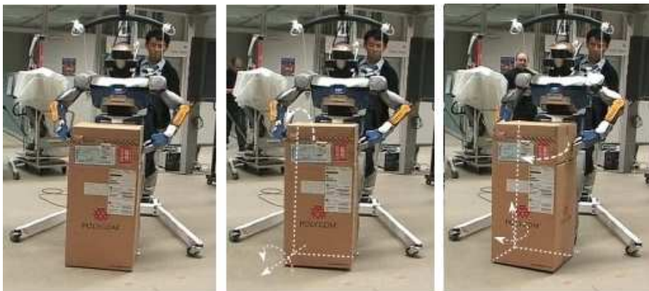
Figure 1.6: From [Yoshida et al. 2007]: HRP-2 is displacing a big wooden box from one location to another by pivoting the object. In this example the motion is precomputed in advance, the locomotion being decoupled from the manipulation.
