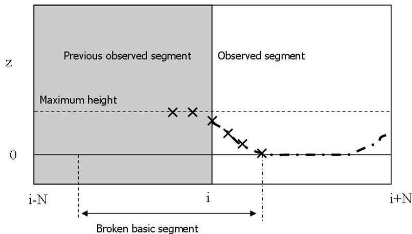
Figure 5.11: Planning the height  $Z$  trajectory. To plan this trajectory we use the information of the basic segment. The via points are represented by cross marks, the observed segment (solid line) is in the white region, while the next segment is in the gray region( dashed line). The thin-horizontal-dashed line indicates the maximum allowed height.
