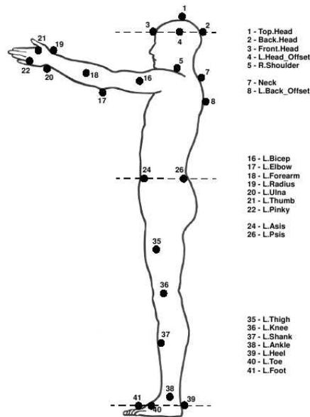
Figure A.5: Marker set left side view.
