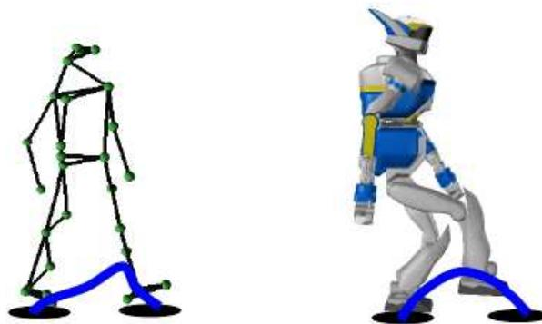
Figure 5.4: Feet motion is planned, it is not imitated directly.
