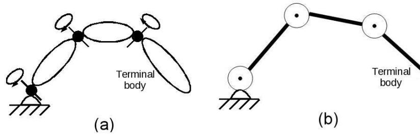
Figure 2.6: (a) A simple manipulator and (b) its geometric model.
