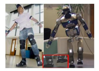
Figure 4.6: Scenario 2. Picture of humanoid imitating the human lifting his foot.
