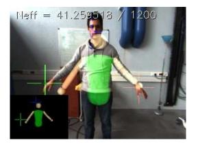
Figure 6.1: A snapshoot of the motion capture system based on stereo vision and particle filtering.
