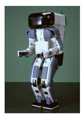
Figure 1.5: P2: the Honda humanoid presented in 1996 that was capable of walking and climbing/descending of stairs. It is 210 kg weight and 182 m height. Picture source http://asimo.honda.com
