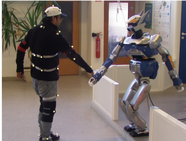
Figure 1.14: Picture of a human performer extending a handshake and the humanoid robot HRP-2 imitating the gesture. The human motion was tracked using reflective motion markers and transferred in real-time to the humanoid.
