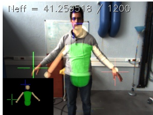
Figure 6.1: A snapshot of the motion capture system based on stereo vision and particle filtering.
