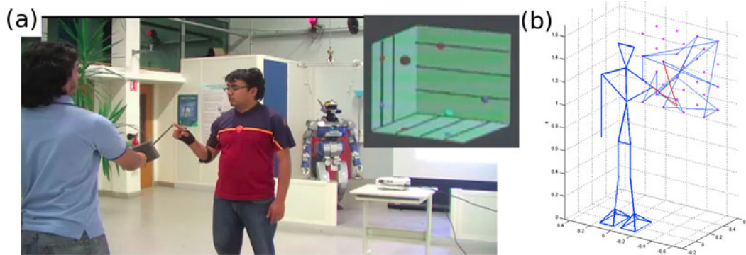
FIGURE 3.6 – (a) Experimental environment : The participants were required to touch a target at the end of a stick with their fingers. The position of the target was manipulated by the experimenter. Inset (right top) shows the current position of the target (green sphere) and the next target (red sphere). Using real-time feedback of the current position the experimenter positioned the stick during the experiment. (b) An illustration of the placement of the virtual grids relative to the participant position. Each participant executed 993 movements such that all 32 targets were reached from each other. Source [Tuan et al. 2010]
