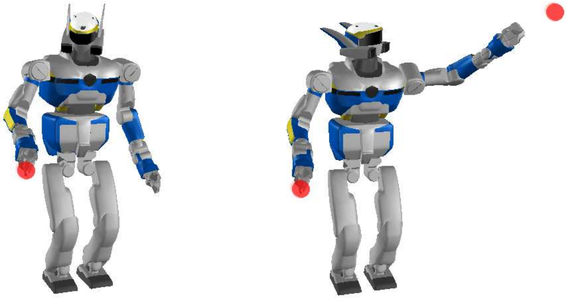
FIGURE 2.2 – Defining multiple tasks for a humanoid robot : Picture of left shows HRP-2 completing two tasks, reach the red target with the right hand and looking at it. On the right we add an additional reaching task for the left hand. In order to avoid conflicts we have to enforce task prioritization.
