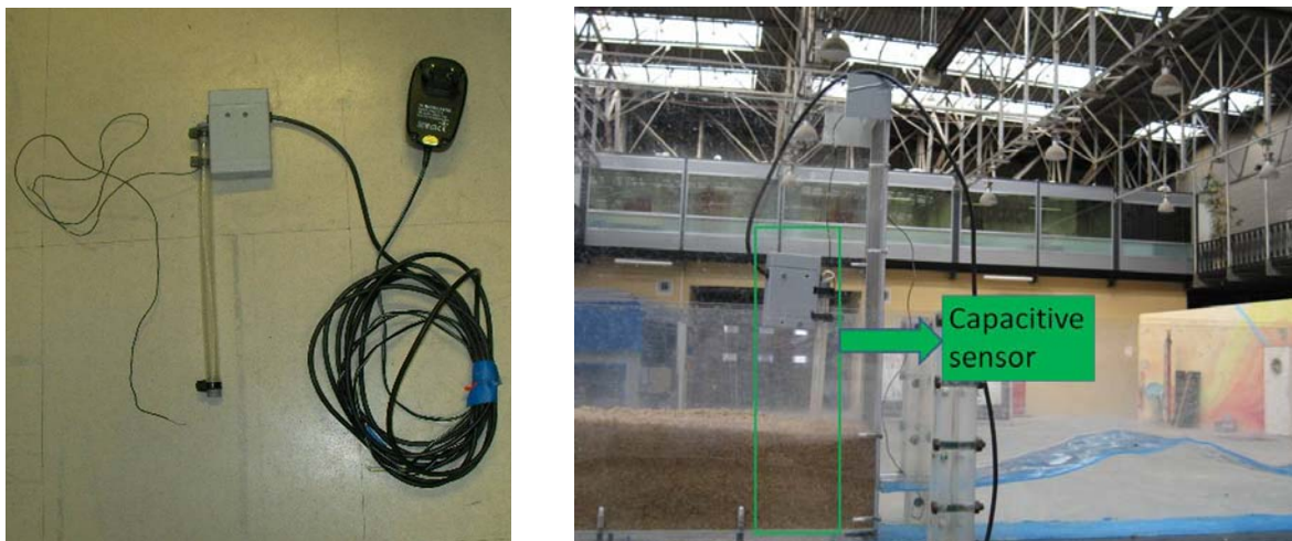
Fig. 4-3 Tested sensors: capacitive sensor used to measure the water level fluctuations in the sandbox
