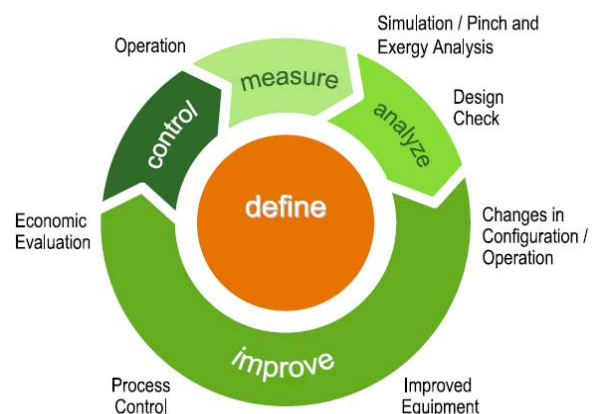
Figure 1.4. Work flow for the analysis of an existing process (Asprion et al. 2011)
