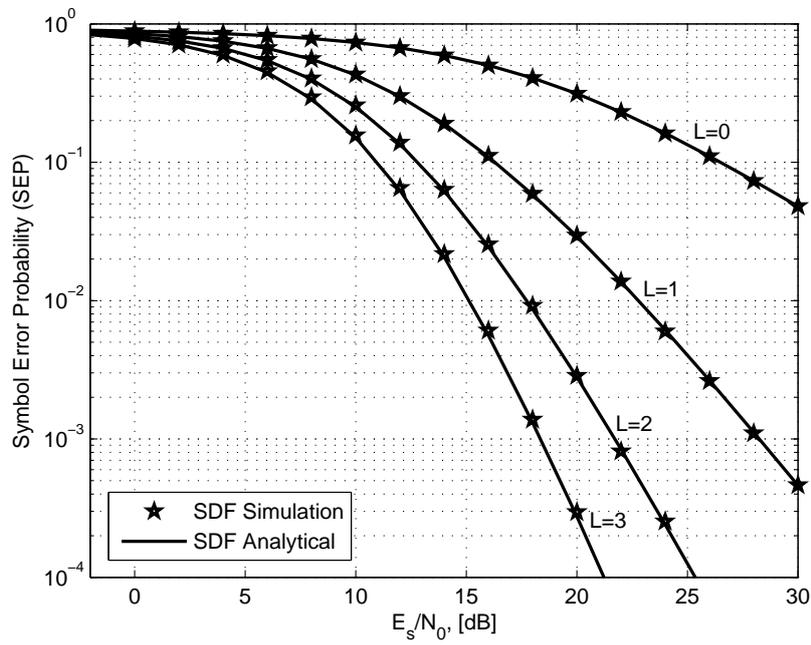
Figure 2.7: The average SEP of a 16QAM HSTCS versus the average transmit SNR,  $E_s/N_0$ , when the direct link experiences the FHS and the satellite-relay links experience the AS and relay-destination links are Rayleigh fading ( $m_{rd} = 1$ ) with the average channel power gain equal to unity.
