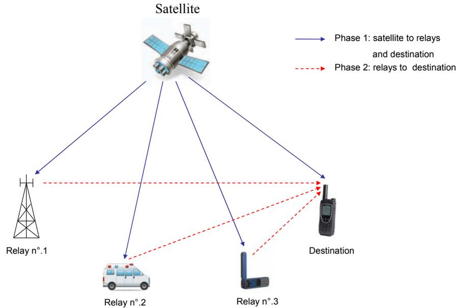
Figure 1.1: HSTCS with 3 relays and one destination.
