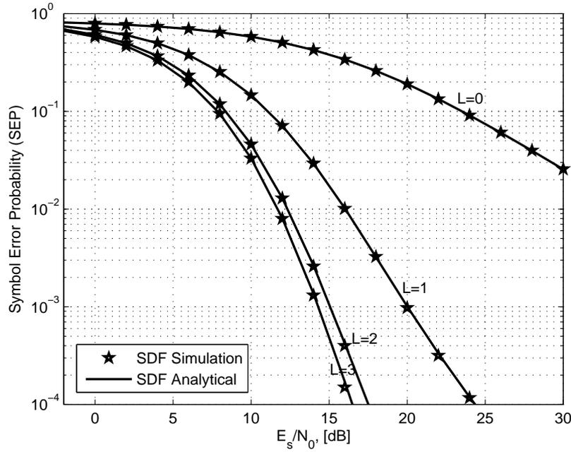
Figure 2.4: The average SEP of a 8PSK HSTCS versus the average transmit SNR,  $E_s/N_0$ , when the direct link experiences the FHS. The first, the second and the third satellite-relay links experience the ILS, the AS and the FHS respectively while their terrestrial links experience the Nakagami- $m$  fading with  $m_{rd}$  equal to 3.5, 5.6 and 1.2 respectively.
