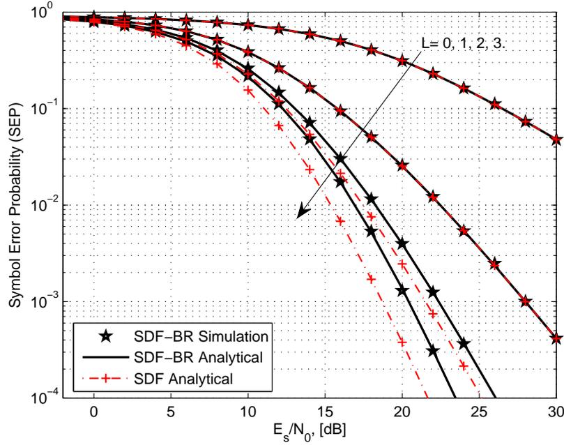
Figure 3.6: The average SEP of a 16QAM HSTCS with best relay selection versus the average transmit SNR,  $E_s/N_0$ , when the direct link experiences the FHS. The first, the second and the third relay experience the ILS, the AS and the ILS respectively while their terrestrial links experience the Rayleigh fading with the average power channel gain equal to 1, 1 and 0.5 respectively.
