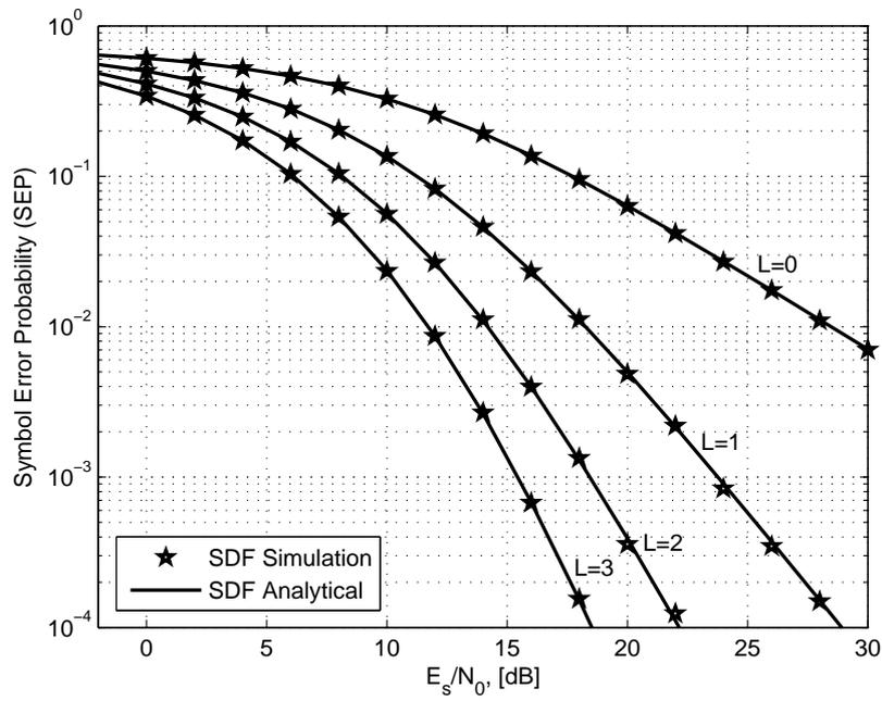
Figure 2.6: The average SEP of a QPSK HSTCS versus the average transmit SNR,  $E_s/N_0$ , when both direct and satellite-relay links experience the FHS and relay-destination links are Rayleigh fading ( $m_{rd} = 1$ ) with the average channel power gain equal to unity.
