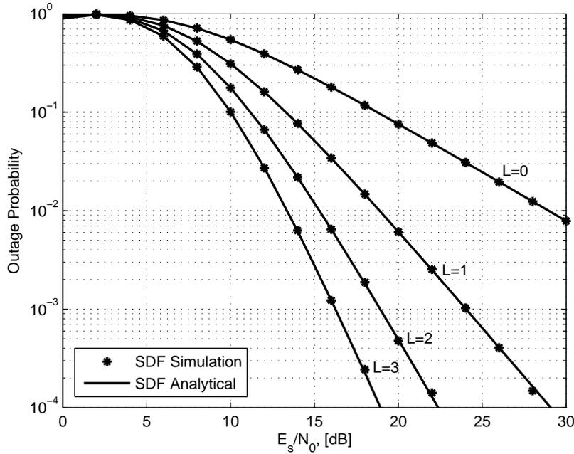
Figure 2.3: The outage probability of an HSTCS versus the average transmit SNR,  $E_s/N_0$ , when both direct and satellite-relay links experience the FHS and the terrestrial links are Rayleigh fading with the average power channel gain equal to unity.
