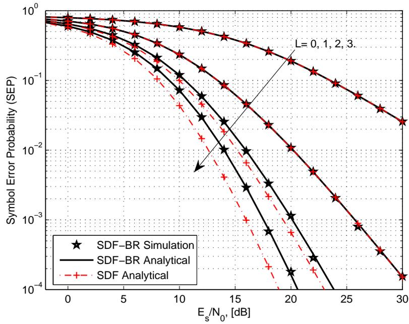
Figure 3.8: The average SEP of a 8PSK HSTCS with best relay selection versus the average transmit SNR,  $E_s/N_0$ , when the direct link experiences the FHS and satellite-relay links experience the AS while their terrestrial links experience the Rayleigh fading with the average power channel gain equal to unity.
