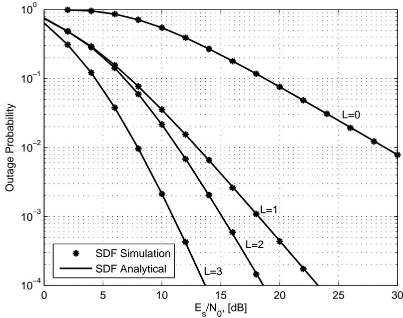
Figure 2.2: The outage probability of an HSTCS versus the average transmit SNR,  $E_s/N_0$ , when the direct link experiences the FHS. The first, the second and the third satellite-relay links experience the ILS, the FHS and the AS respectively while their terrestrial links experience the Rayleigh fading with the average power channel gain equal to 1, 0.25 and 0.5 respectively.
