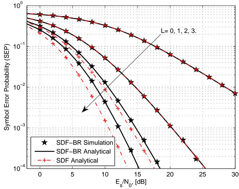
Figure 3.7: The average SEP of a QPSK HSTCS with best relay selection versus the average transmit SNR,  $E_s/N_0$ , when the direct link experiences the FHS and satellite-relay links experience the AS while their terrestrial links experience the Rayleigh fading with the average power channel gain equal to unity.
