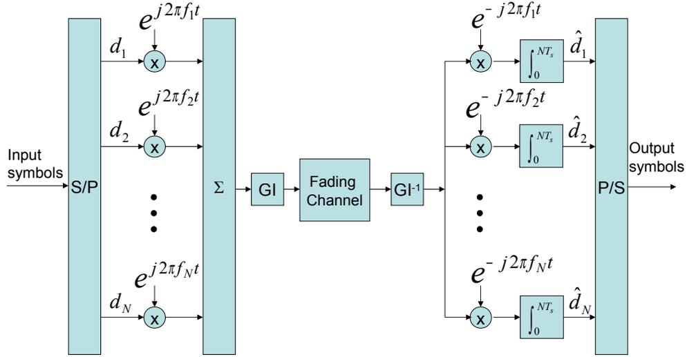
Figure 4.1: Base-band OFDM system model with  $N$  subcarriers.
