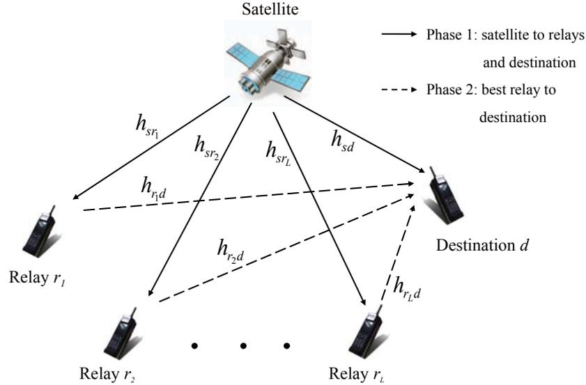
Figure 3.1: Hybrid satellite-terrestrial system with  $L$  relays and one destination.
