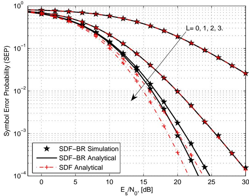
Figure 3.5: The average SEP of a 8PSK HSTCS with best relay selection versus the average transmit SNR,  $E_s/N_0$ , when the direct link experiences the FHS. The first, the second and the third relay experience the ILS, the AS and the FHS respectively while their terrestrial links experience the Rayleigh fading with the average power channel gain equal to 1, 0.5 and 0.25 respectively.
