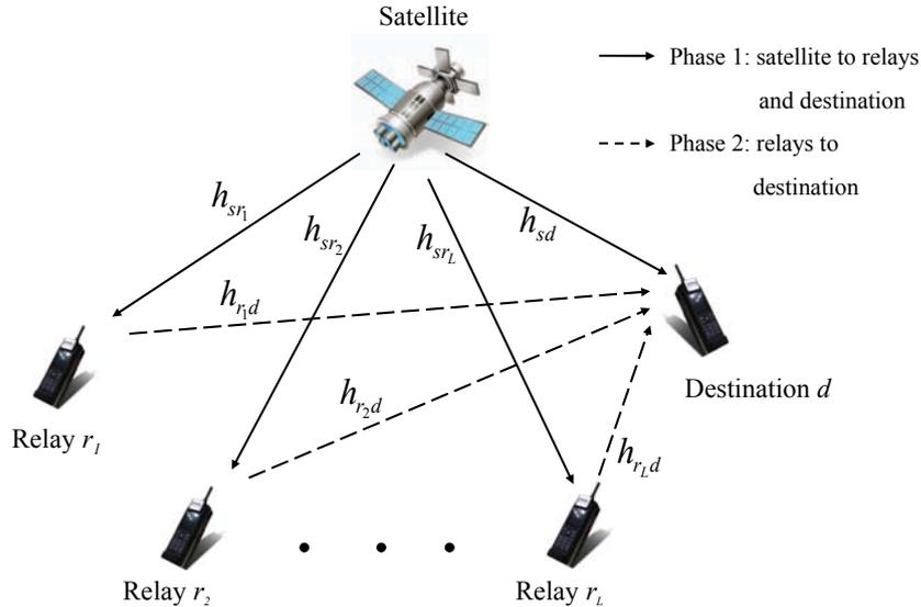
Figure 2.1: Hybrid satellite-terrestrial system with  $L$  relays and one destination.
