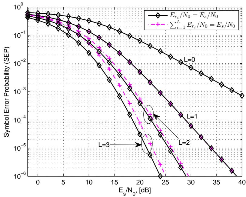
Figure 2.8: The analytical SEP of a QPSK HSTCS with different transmit SNR,  $E_{r_i}/N_0$ , scenarios, when both direct and satellite-relay links experience the FHS and relay-destination links are Rayleigh fading ( $m_{rd} = 1$ ) with the average channel power gain equal to unity.
