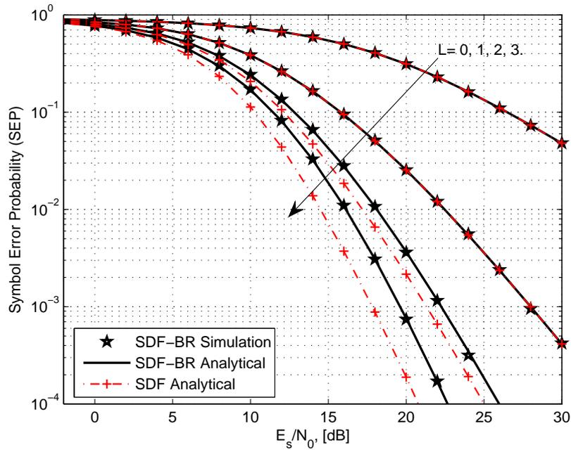
Figure 3.9: The average SEP of a 16QAM HSTCS with best relay selection versus the average transmit SNR,  $E_s/N_0$ , when the direct link experiences the FHS and the satellite-relay links experience the ILS while their terrestrial links experience the Rayleigh fading with the average power channel gain equal to unity.
