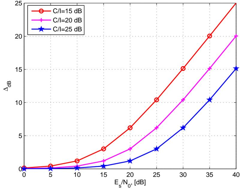
Figure 4.4: Degradation  $\Delta_{dB}$  as a function of  $E_s/N_0$ .
