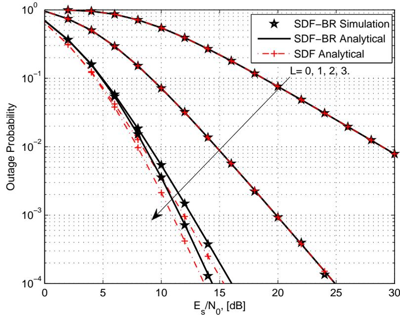
Figure 3.2: The outage probability of an HSTCS with best relay selection versus the average transmit SNR,  $E_s/N_0$ , when the direct link experiences the FHS. The first, the second and the third satellite-relays experience the AS, the ILS and the FHS respectively while their terrestrial links experience the Rayleigh fading with the average power channel gain equal to 0.5, 1 and 0.25 respectively.
