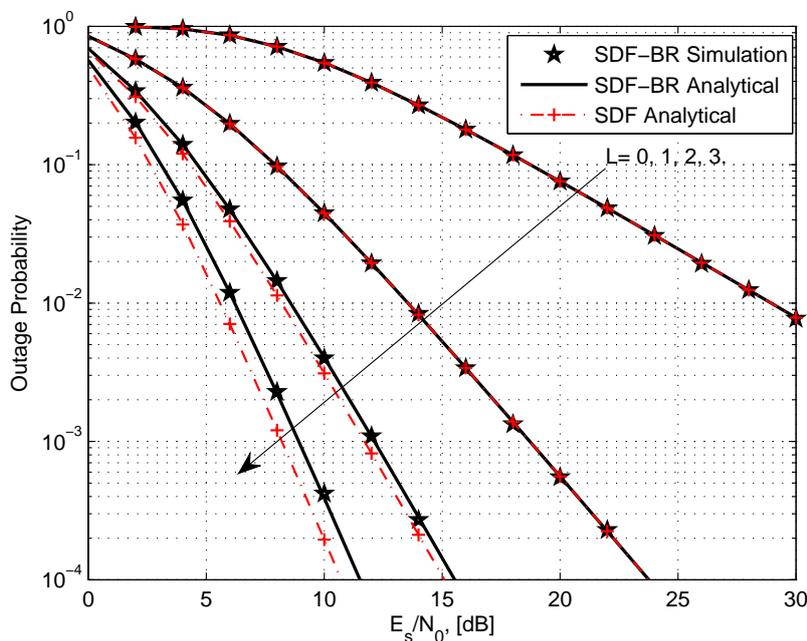
Figure 3.3: The outage probability of an HSTCS with best relay selection versus the average transmit SNR,  $E_s/N_0$ , when the direct link experiences the FHS and the relay links experience the AS while their terrestrial links experience the Rayleigh fading with the average power channel gain equal to unity.
