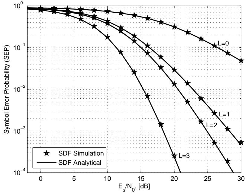
Figure 2.5: The average SEP of 16QAM HSTCS versus the average transmit SNR,  $E_s/N_0$ , when the direct link experiences the FHS. The first, the second and the third satellite-relay links experience the AS, the FHS and the ILS respectively while their terrestrial links experience the Nakagami-m fading with  $m_{rd}$  equal to 1, 0.5 and 2.8 respectively.
