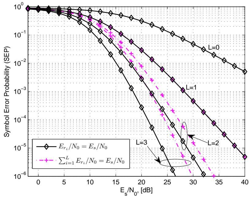
Figure 2.9: The analytical SEP curves of a 16QAM HSTCS with different transmit SNR,  $E_{r_i}/N_0$ , scenarios, when the direct link experiences the FHS and the satellite-relay links experience the AS and relay-destination links are Rayleigh fading ( $m_{rd} = 1$ ) with the average channel power gain equal to unity.
