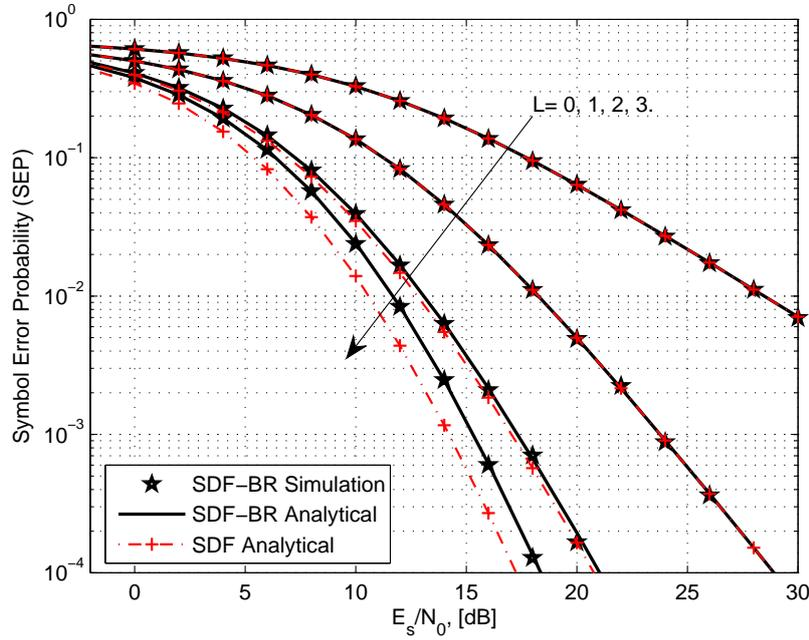
Figure 3.4: The average SEP of a QPSK HSTCS with best relay selection versus the average transmit SNR,  $E_s/N_0$ , when the direct link experiences the FHS. The first, the second and the third relay experience the FHS, the AS and the ILS respectively while their terrestrial links experience the Rayleigh fading with the average power channel gain equal to 1, 0.5 and 0.25 respectively.
