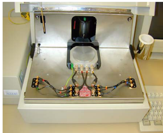
Figure 63: HL5500PC Hall Effect Measurement System.
