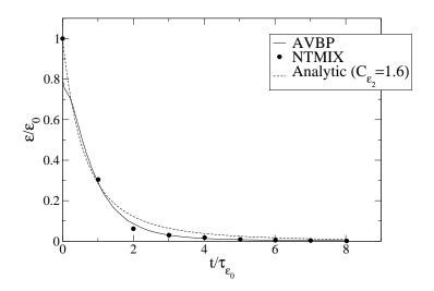
Figure 2.3: Comparison of the evolution of dissipation between AVBP, NTMIX and analytical predictions from  $k - \epsilon$  model.  $C_{\epsilon_2}$  is chosen to 1.6 which is a typical value for low resolution DNS
