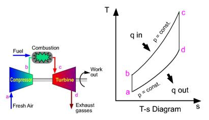
Figure 1.2: Thermodynamic cycle of gas turbine engines
