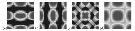
Figure 8.23: Nearest neighbor results for different meshes: (a) 51x49, (b) 49x51, (c) 49x49, (d) 51x51
