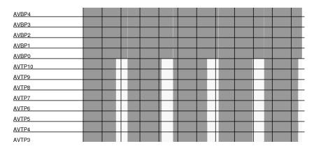
Figure 12.7: A portion of the Gant diagram of a well balanced coupled application. The white areas represent processors waiting, the gray areas represent active processors. Each cell corresponds to 5s
