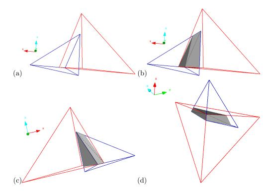
Figure B.8: Demonstration of the intersection of two tetrahedra. Two tetrahedra are presented in (a), their intersection polyhedron is computed by first computing the intersection points and then using incremental hull. Different views of the tetrahedrons and their intersection polyhedron are showed in (b),(c) and (d).
