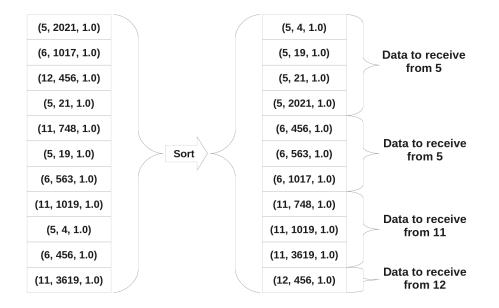
Figure 13.8: Construction of the reception vector by sorting the data sources
