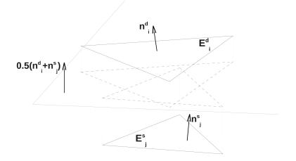
Figure 9.3: Before calculating the intersection polygons the source and destination elements are projected on a average plane
