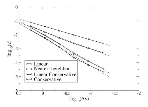
Figure 8.19: Error comparison of interpolation methods
