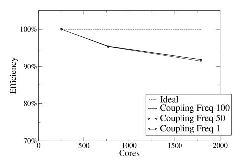
Figure 14.3: LES solver efficiency for different coupling frequencies
