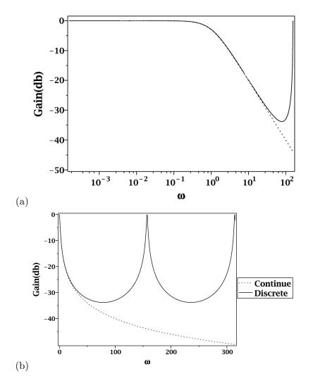
Figure 6.4: Comparison between the continuous and the discrete low pass/integrator filter: (a) on a  $[0, \omega_s]$  period on a log-log diagram, (b) on  $[0, 2\omega_s]$  on a semi-log diagram.
