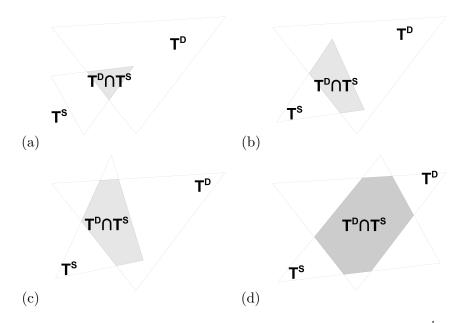
Figure 9.4: Examples of intersections between destination and source triangles  $T^d$  and  $T^s$ : (a) 3 point intersection, (b) 4 point intersection, (c) 5 point intersection, (d) 6 point intersection
