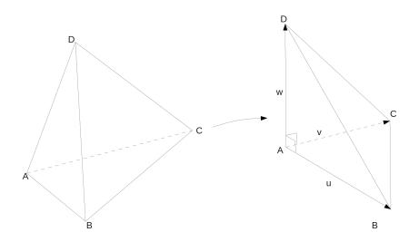
Figure B.6: Calculating an integral on a tetrahedron
