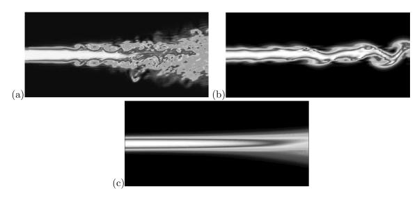
Figure 1.6: Comparison of flames using DNS (a), LES (b), RANS (c)
