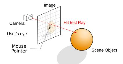
Figure A.7: Process to do a hit test from a user click: user clicks on a 2D image the search is performed in a 3D space using a hit test ray
