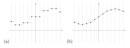
Figure 8.10: The reconstructed signal: (a) box filter, (b) tent filter
