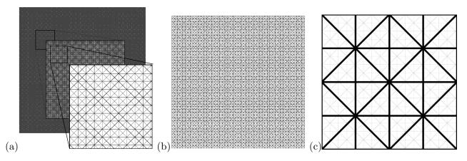
Figure 8.20: (a) Fine grid(200x200), (b) coarse Grid(51x49), (c) a section of the fine and coarse grids overlapped.
