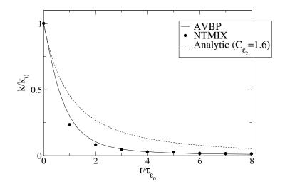
Figure 2.4: Comparison of the evolution of kinetic energy between AVBP, NTMIX and analytical predictions from  $k - \epsilon$  model.  $C_{\epsilon_2}$  is chosen to 1.6 which is a typical value for low resolution DNS
