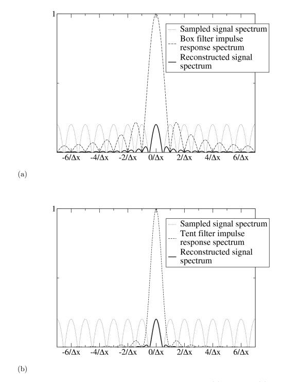
Figure 8.14: Frequency view of signal reconstruction using: (a) box filter, (b) tent filter
