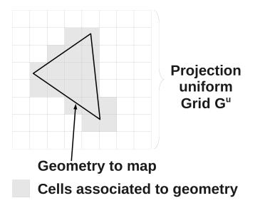
Figure 13.4: Geometry projection to cell list
