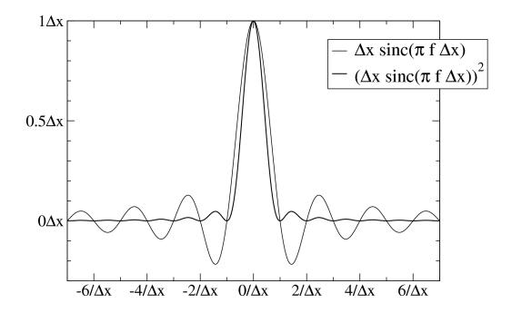
Figure 8.13: Comparisons of the Fourier transform of the tent and box filter's impulse response
