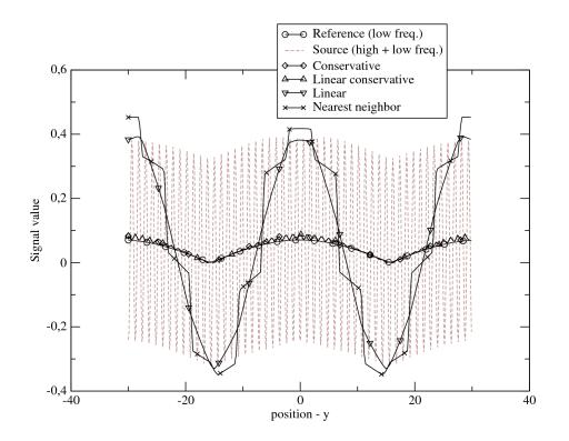
Figure 8.29: Interpolation profile on line x = 15
