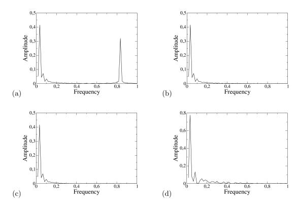
Figure 8.31: x = 0 profile spectrum for different signals: (a) Source (low+high freq.), (b) Low frequency reference, (c) Linear conservative, (d) Nearest neighbor
