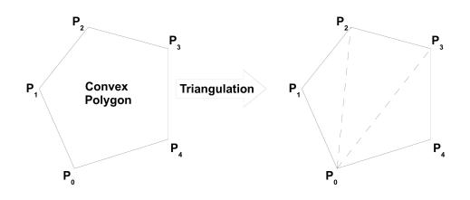
Figure 9.7: Triangulating a convex polygon into a triangle fan
