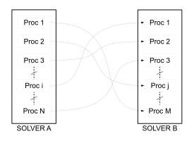
Figure 11.4: Direct Communication scheme(DCS)
