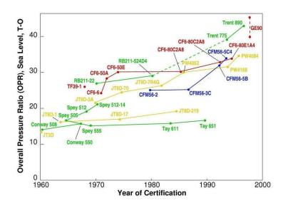
Figure 1.3: Gas turbine engine pressure ratio trends (www.mit.edu - Jane's Aeroengines, 1998)
