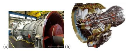
Figure 1.5: (a) An industrial gas turbine(Siemens), (b) The cfm-56 Turbofan Engine (Snecma)
