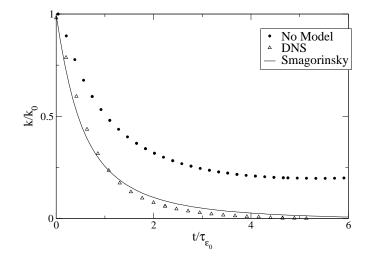
Figure 2.5: Comparison of LES and DNS on a HIT case
