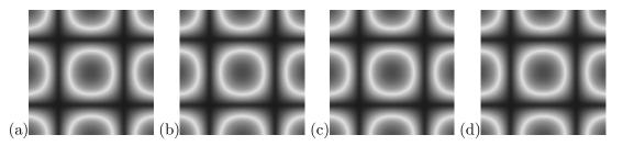
Figure 8.25: Linear conservative interpolation results for different meshes: (a) 51x49, (b) 49x51, (c) 49x49, (d) 51x51
