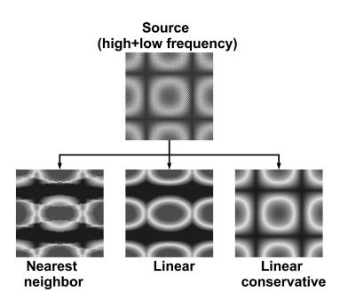
Figure 8.22: Interpolation from fine to coarse grid
