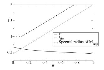
Figure 7.4: This graph shows two stability conditions together we can see that when  $r > r_{max}$ ,  $\rho(M) > 1$ .
