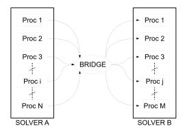
Figure 11.3: Centralized Communication scheme (CCS)
