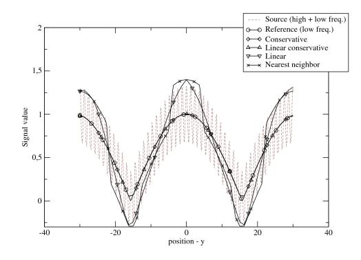
Figure 8.27: Interpolation profile on line x = 0
