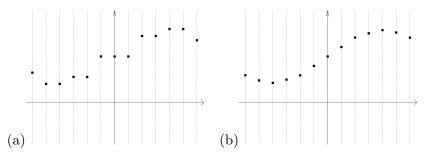
Figure 8.11: The sampled signal on destination grid: (a) box filter, (b) tent filter
