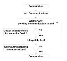
Figure 13.10: Communication algorithm with overlapped interpolation
