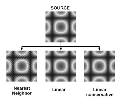
Figure 8.21: Interpolation from coarse to fine grid
