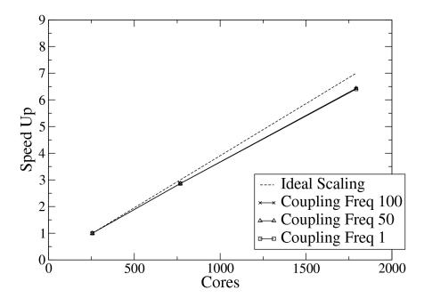
Figure 14.2: LES solver scalability curve for different coupling frequencies. Coupling Freq. 50 means that 50 LES iterations are executed between two coupling updates. Coupling Freq. 1 means that a couling update is done at each LES iteration.
