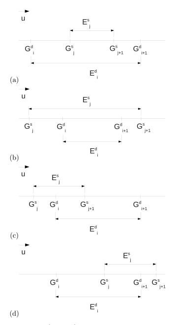
Figure 8.17: (a)  $E_j^s$  is contained in  $E_i^d$ , (b)  $E_i^d$  is contained in  $E_j^s$ , (c)  $E_j^s$  has intersection with  $E_i^d$  on its left, (d)  $E_j^s$  has intersection with  $E_i^d$  on its right
