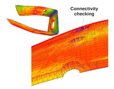
Figure A.2: Basic visual connectivity checker associated to the interpolator
