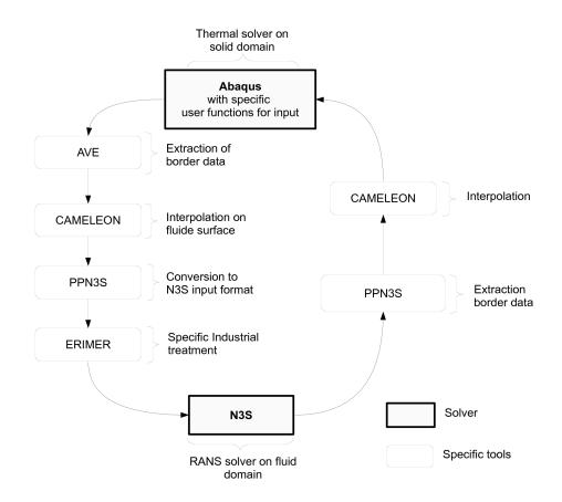
Figure 1.11: N3S-ABAQUS Coupled chain developed at Snecma
