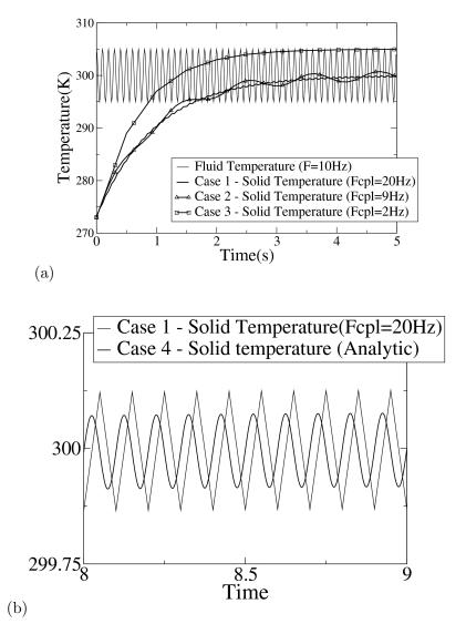
Figure 6.2: Evolution of solid temperature in loose coupling environment: (a) cases 1, 2, 3 and 4 (b) comparison of 1 and 4
