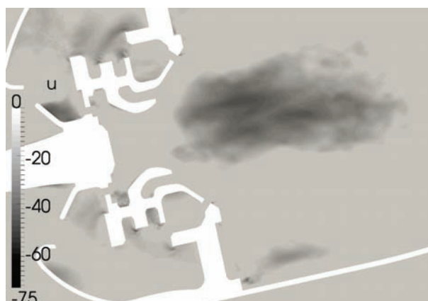
Figure 4.16: Negative axial velocity region inside the central recirculation zone
