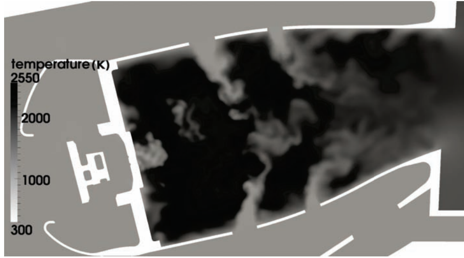
Figure 4.20: Instantaneous temperature field in the flame tube (Cut2)
