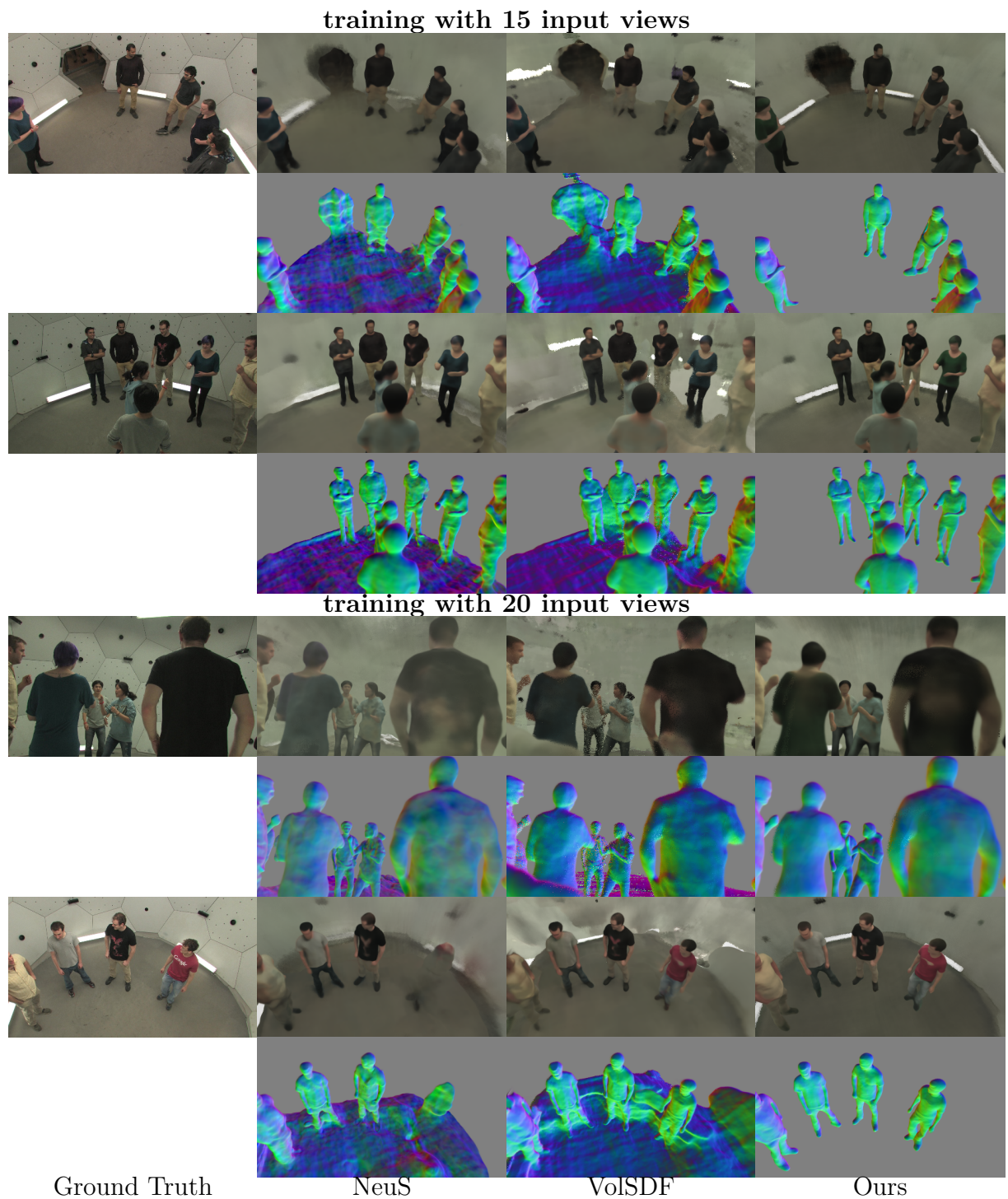
Figure 5.6 – Qualitative comparison against NeuS [34] and VolSDF [77] of synthesized novel views and reconstructed normal images of multiple humans on CMU Panoptic dataset [1], [2], using 15/20 training views.
