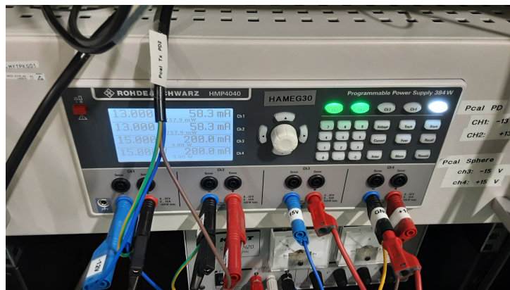
Figure 5.8: Picture of front panel of Rohde&Schwartz HMP4040 voltage generator.
