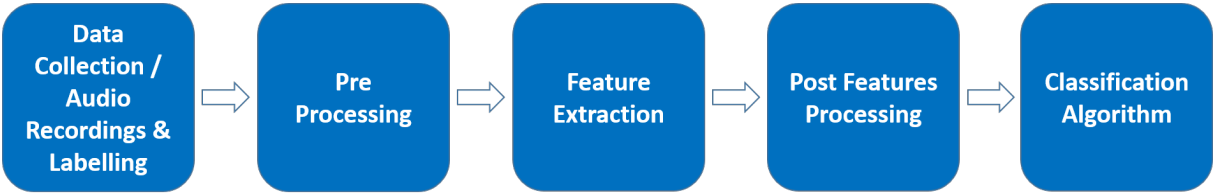
Figure 2 – Environmental sound classification system block diagram.
