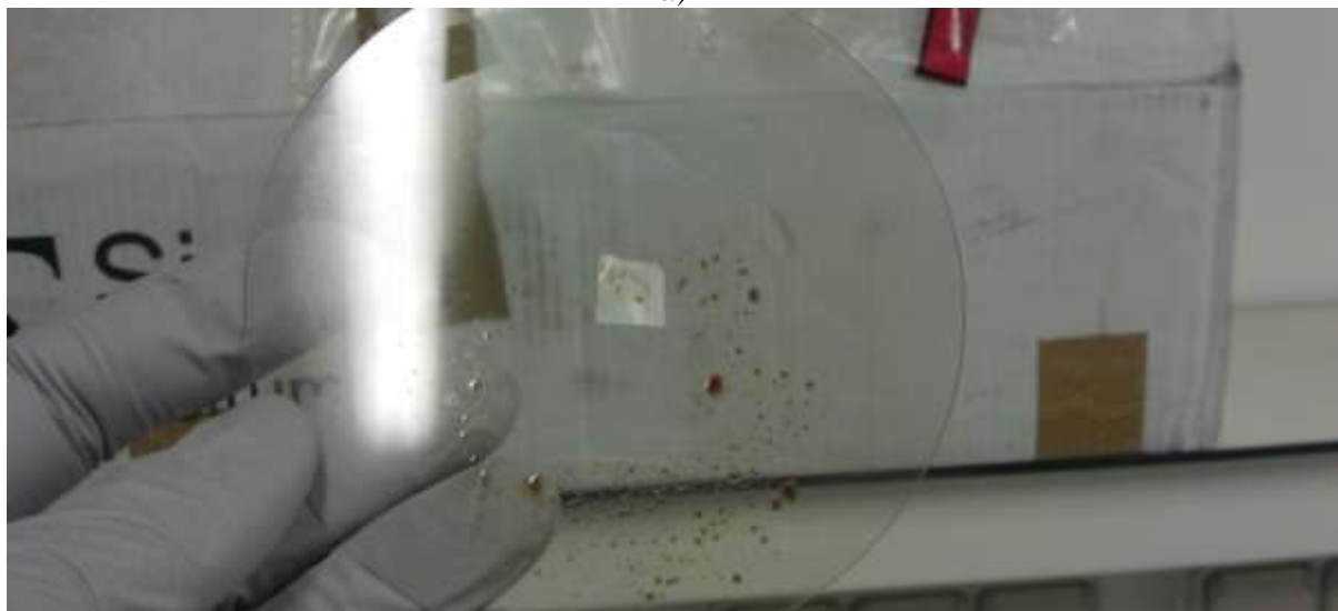
Figure 4.2: The substrates after the deposition a) noted as P1.1 glass, P1.2 Si(111), P1.3 SiO x /Si(100), P1.4 Si(111) and b) the substrates glass holder with the deposited droplets one week later
