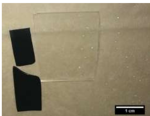
Figure 3.2: The samples obtained after the Photo-CVD deposition (experimental data in Table 3.1)
