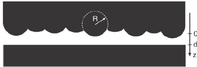
Figure 2.3: Greenwood & Williamson contact theory between a smooth plane and a rough surface. All asperities with height z greater than the separation d make contact [8].
