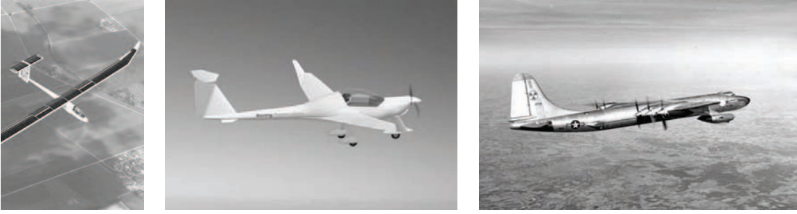
Figure 1.1: Examples for non-combustion based aeronautical concepts. Left: Icaré solar aircraft (photo Universität Stuttgart). Center: Boeing phantom works fuel cell demonstrator (Photo: Boeing). Right: Convair NB-36H nuclear testbed (Photo: Wikipedia).
