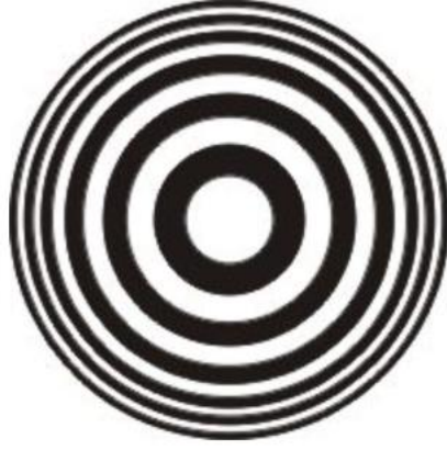
Figure 2.15: Illustration of the Fresnel Zone Plate
