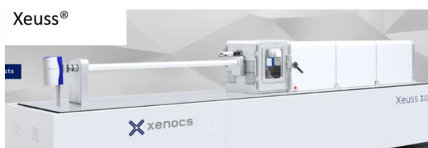
Figure 6.1: (a) The newly available SAXS/WAXS laboratory equipment and (b) the 2D composite image in GIWAXS mode (incident angle of 5^\circ ) of a PZT 30/70 1 \mu\text{m} film where multiple Debye rings are collected
