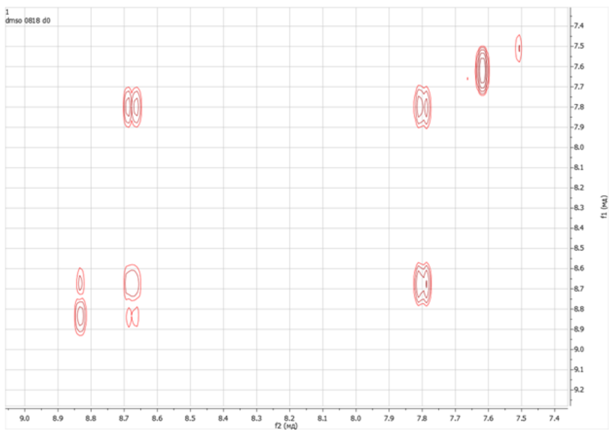
Figure A14: ^1\text{H} - ^1\text{H} COSY NMR spectrum of 2,4,5,7,4'-pentanitrofluorescein (400 MHz, DMSO- d_6 ).
