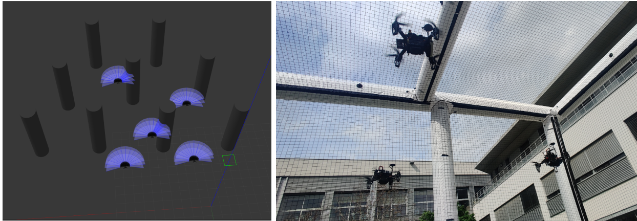
Figure 7.1: a. Snapshot of 5 IntelAero drones flocking together with the VAT model in the GAZEBO simulator b. Experiment of a 3-drones flocking by the Chroma team on April 2023 (CITI lab.)
