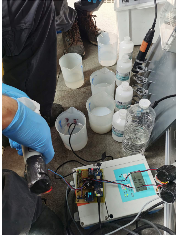
Figure 12. Turbidimeter in field calibration.
