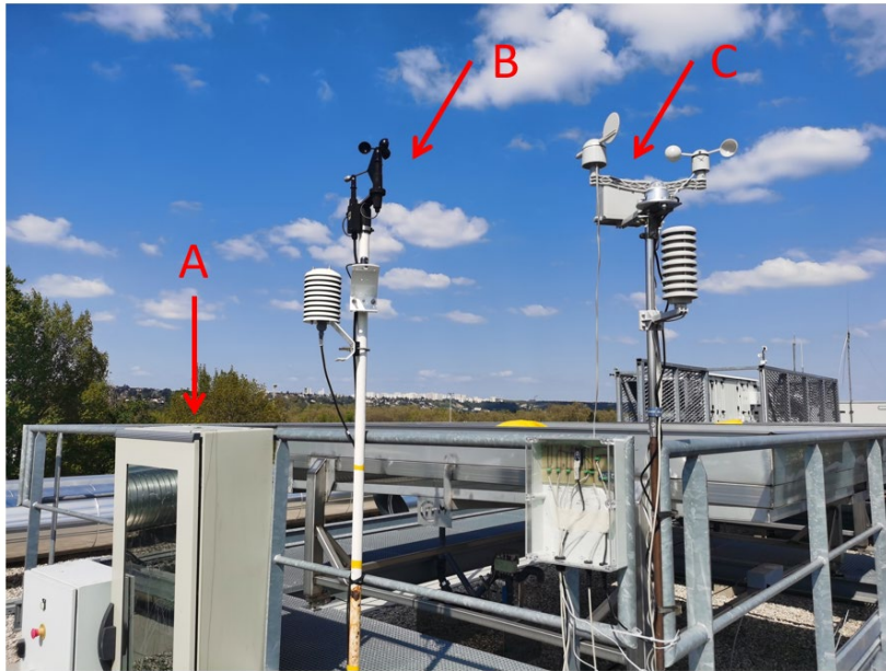
Figure 4-14. One side view of low-cost and reference meteorological sensors installation with the waterproof cabinet (A), the reference weather station (B), and the low-cost weather station (C).
