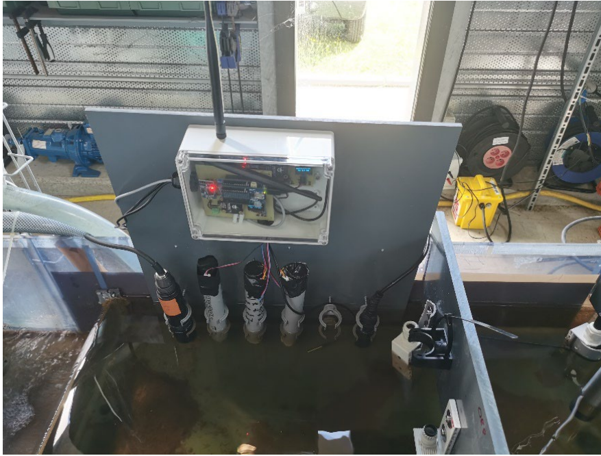
Figure 11. Installation of low-cost and reference turbidimeters on 2022-07-22, add a reference DIY data logger and screens on data loggers. A shade to reduce the effects of sunlight.
