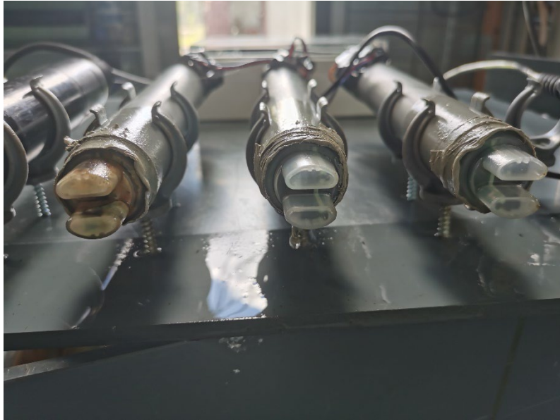
Figure 7. Water enters one DIY turbidimeter probe (the left one).
