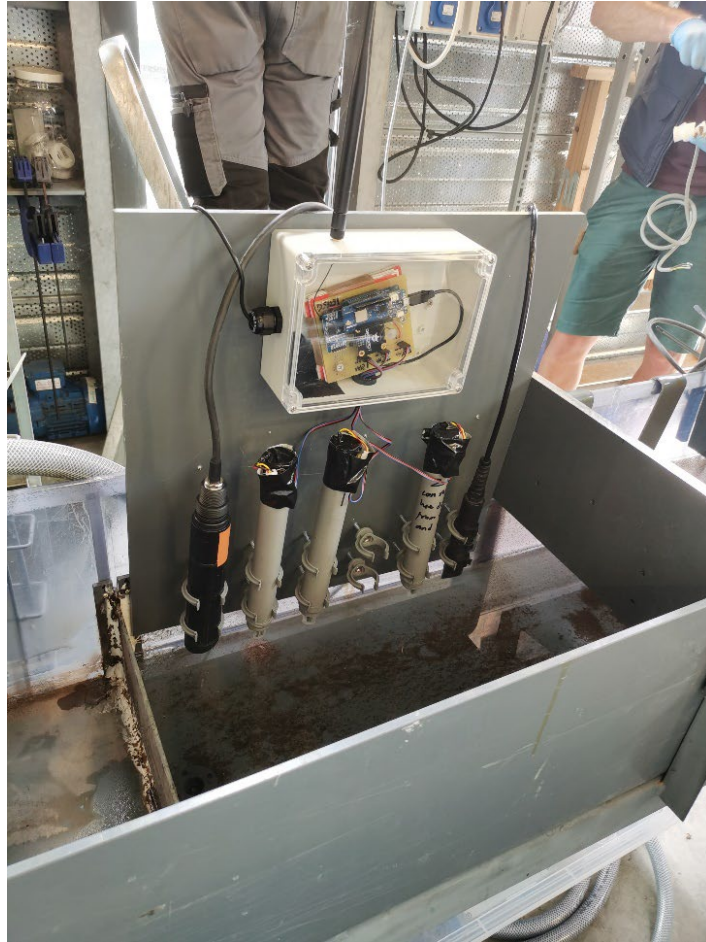
Figure 10. Turbidimeters first test setups on 2022-05-12. Low-cost data logger is in the box on the top. Turbidimeters are on the bottom: from left to right, reference sensor Turbimax W CUS41, low-cost sensor No. 1 to 3 and reference Aqualabo sensor.
