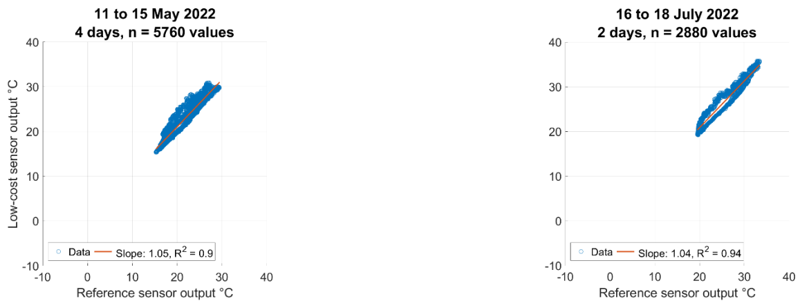
Figure 4-27. Comparison between DHT22 and reference sensor air temperature measurements in May and July 2022.
