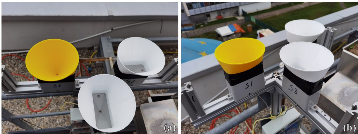
Figure 5-40. New test setups: new additional enlarged funnel in conical shape in yellow color installed on low-cost TBRG No.4 and old additional enlarged funnel in white color installed on low-cost TBRG No.5 and No.6. (a) Top view, (b) Side view.
