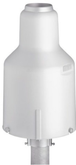
Figure 3-8. Picture of the OTTPluvio 2 L rain gauge. Source: ott.com (accessed: 29 March 2023).
