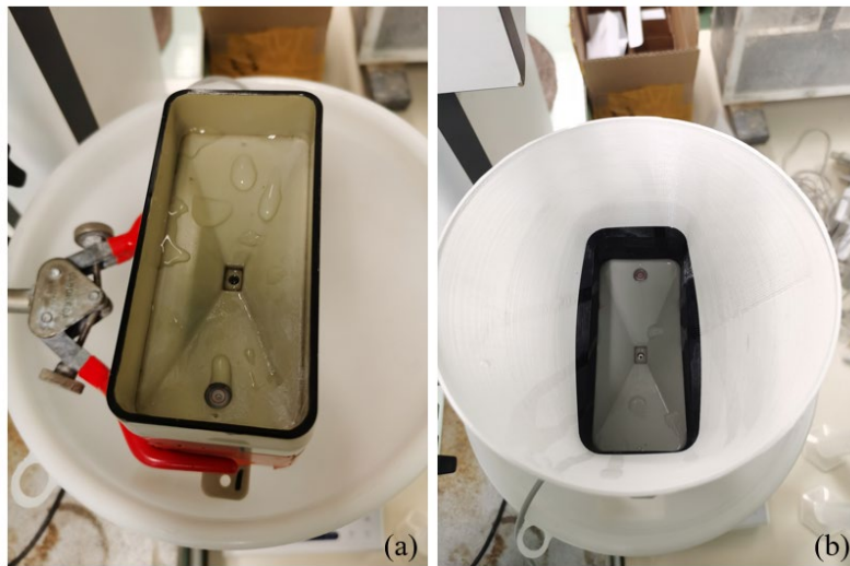
Figure 5-38. Water drops cannot flow easily on WH-SP-RG. (a) TBRG No.1 with initial funnel, (b) TBRG No.4 with the first version of the additional enlarged funnel.
