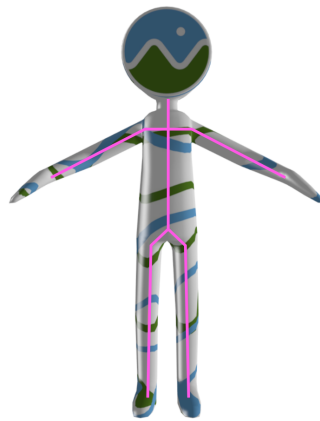
FIGURE 2.1: A textured 3D mesh with its underlying animation skeleton (in pink).
