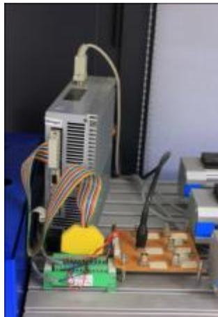
Figure B.2: Variable speed drive SEC-AC-305 (Festo)
