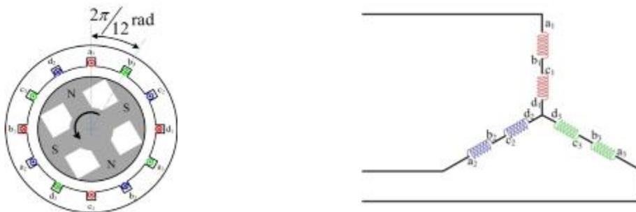
Figure 2.3: Stator windings of a three-phase PMSM 2 pole pairs
