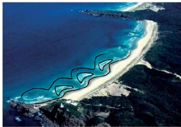
Figure 1.6: Aerial photography of the coupled morphologies between the intertidal and subtidal areas. Shoreline oscillations are coupled to the sand bars geometry. Illustration adapted from (Price et al., 2013).
