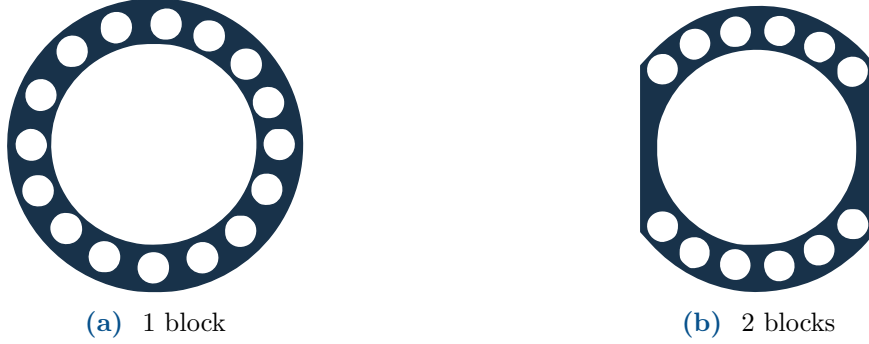
Figure C.2: Types of motor blocks. (a) Ventilation system composed of a single block. (b) Truncated ventilation system composed of two blocks.
