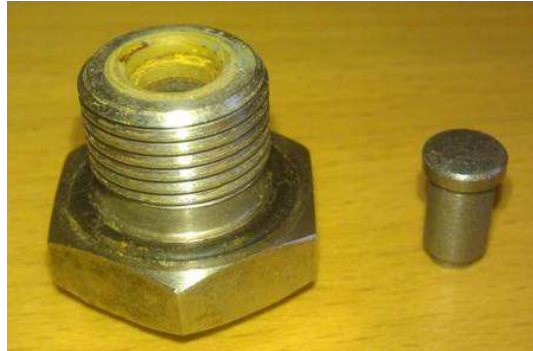
Fig. III. 6. Bio-stud installed in modified-robbins device.
