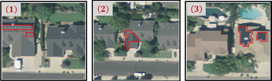
Figure 1.11. The examples of PV detection are based on very high-resolution color satellite imagery [35]
