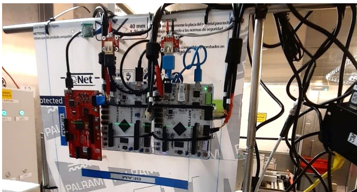
Figure 111: Neutron test setup. The three FPGA boards are mounted on a plexiglass board and aligned with the neutron beam spot. IGLOO2 board on the left, Spartan7 board in the middle and Artix7 on the right.
