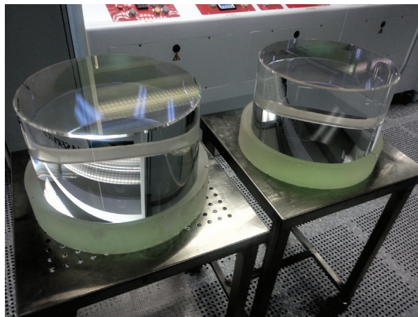
Figure 2.7: Pictures of Advanced Virgo substrates in the cleanroom of LMA after polishing and before coating. Crédit LMA/CNRS.
