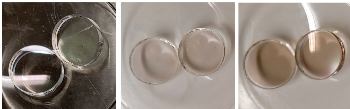
Figure 4.18: Pictures of the samples at the exit of the coating chamber. At 100°C the samples are transparent but at 200°C and 300°C the samples are more and more brownish.
