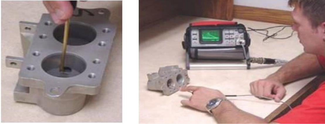
Figure 1-11: Operator testing a mechanical spare part using an eddy current probe[56]
