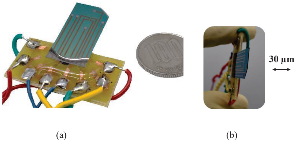
Figure 2-24: PMNP/GMR 2-in-1 sensor; (a) view of the entire sensor; (b) zoom on the thickness of the sensor
