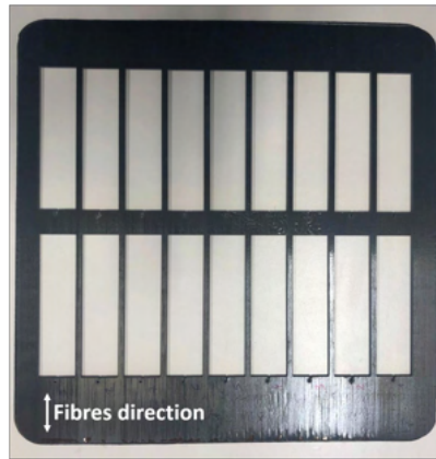
Figure 2.17: Abrasive water-jet cutting of 300 x 300 mm^2 APC-2 plate
