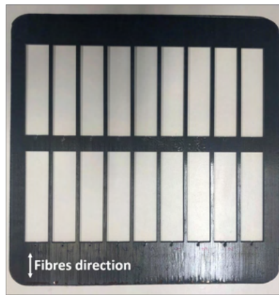
Figure 2.17: Abrasive water-jet cutting of 300 \times 300 \text{ mm}^2 APC-2 plate
