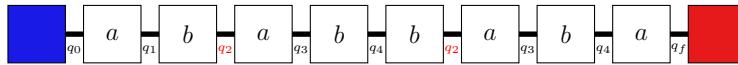
Figure 1.2: A set of dominos generated from the finite automaton of Figure 1.1. We represent the terminal assemblies corresponding to the words ababa and ababbaba . Note that for the second terminal assembly, the glue q_2 (in red) appears two times and the tiles between these two glues can be pumped.
