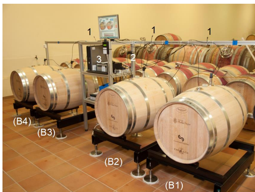
Figure 2-2: Overview of the experimental device installed in the cellar of Château Phélan Ségur. (1) Sensirion sensors; (2) Pressure sensor; (3) Data acquisition system; (Bi) Barrel #i.
