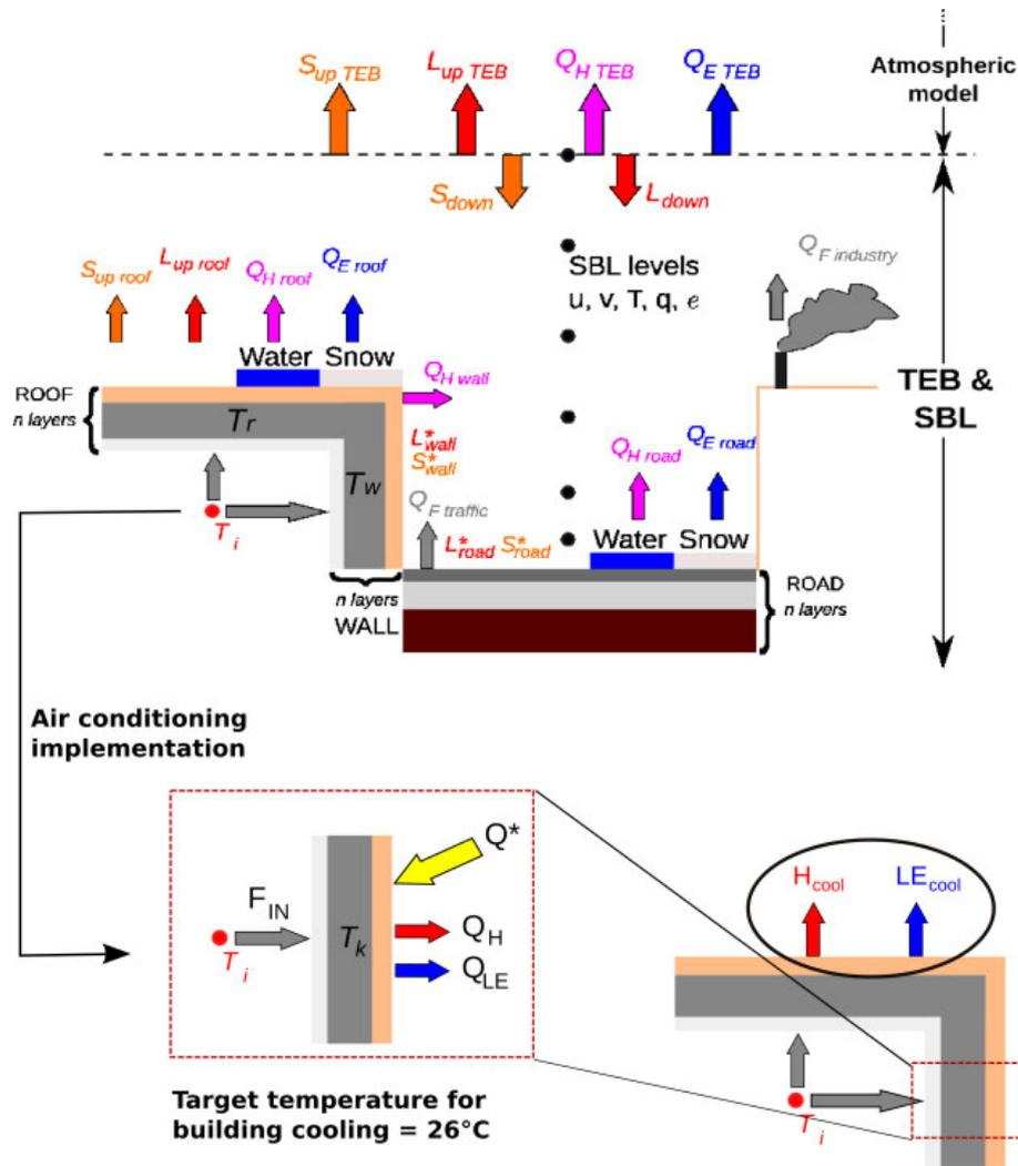
Figure 3. Schematic description of TEB model, showing how AC is accounted for at the building level. This figure is available in colour online at [wileyonlinelibrary.com/journal/joc](http://wileyonlinelibrary.com/journal/joc)
