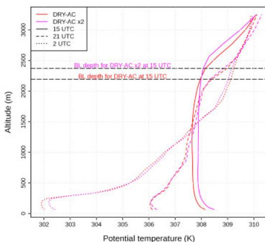
Figure 9. Vertical profile of potential temperature (averaged across a  $2.5 \times 2.5 \text{ km}^2$  zone centred on the west-to-east cross-section shown in Figure 7) for the DRY-AC and the DRY-ACx2 scenarios, on 10/08/2003 15 and 21 UTC and 11/08/2003 2 UTC. This figure is available in colour online at [wileyonlinelibrary.com/journal/joc](http://wileyonlinelibrary.com/journal/joc)
