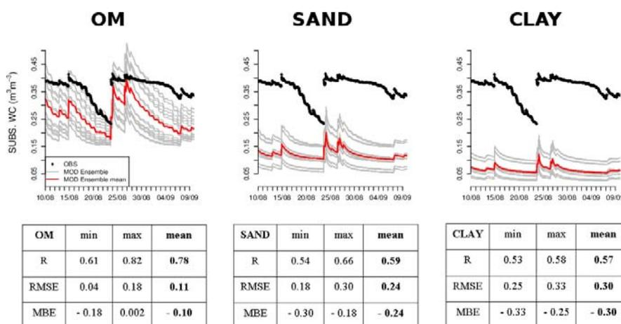
**Fig. 5.** Comparison of the three ensemble simulations OM, SAND and CLAY with regard to their ability to model substrate water content over the calibration period (10 August 2011–9 September 2011). Graphs represent the evolution of the water content with time for each ensemble, while the tables gather their respective scores.  $R$  is the correlation coefficient (–), RMSE the root-mean-square error and MBE the mean bias error ( $\text{m}^3 \text{ m}^{-3}$ ).
