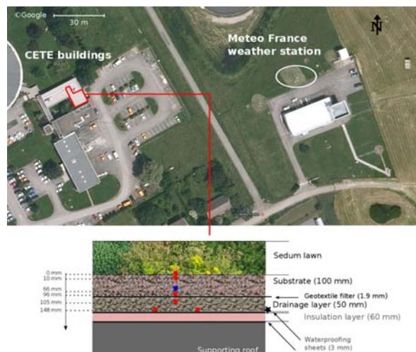
**Fig. 3.** Location (top) and design (bottom) of the green roof experimental plot modelled, showing the positions of the various sensors (red squares for temperature sensors, blue circle for water content and matrix potential sensor and star for drainage water gauge).
