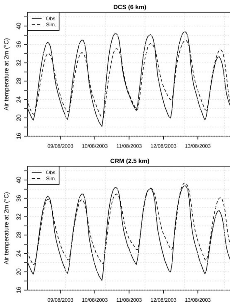
Figure A2. Mean (across 63 weather stations) 2-m air temperatures observed and simulated with a Deep Convection Scheme (DCS) configuration running at a 6 km spatial resolution (top) and with a Cloud Resolving Model (CRM) running at a 2.5 km spatial resolution (bottom), between the 8 and 14 of August 2003.
