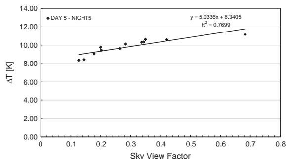
Fig. 11. Absolute temperature swing between the average temperature of the fifth day and the fifth night of the heat wave for the REAL scenario and the 12 meshes versus their sky view.
