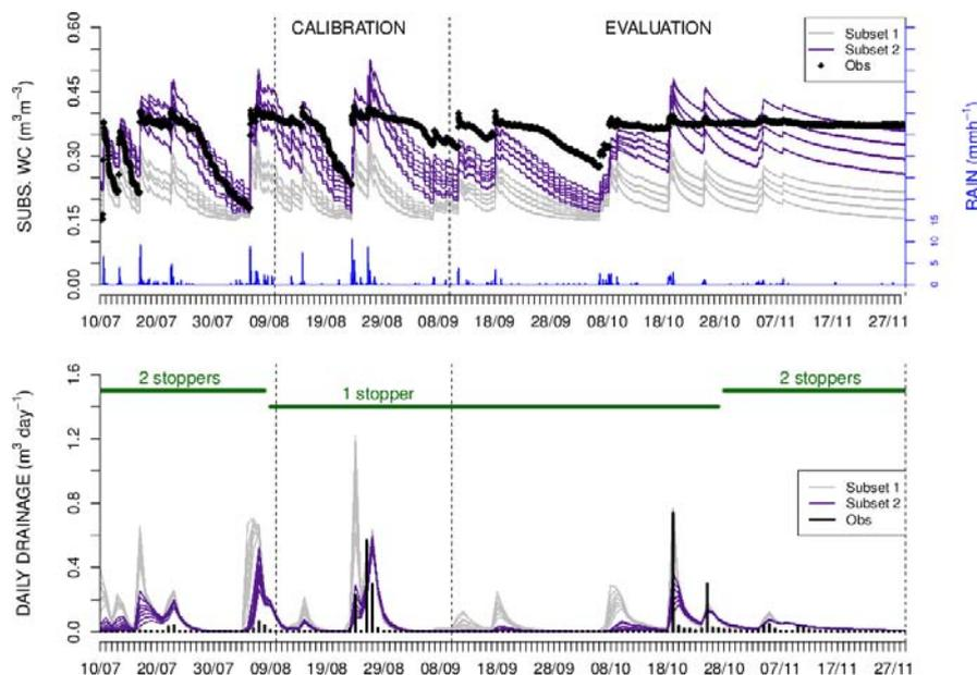
**Fig. 7.** Evolution between 10 July 2011 and 29 November 2011 of SUBSTRATE water content (top) and daily outlet DRAINAGE (bottom), as observed and simulated by the GREENROOF OM ensemble. Rain amount recorded during the experiment is represented by blue bars (right-hand-side axis on top graph).
