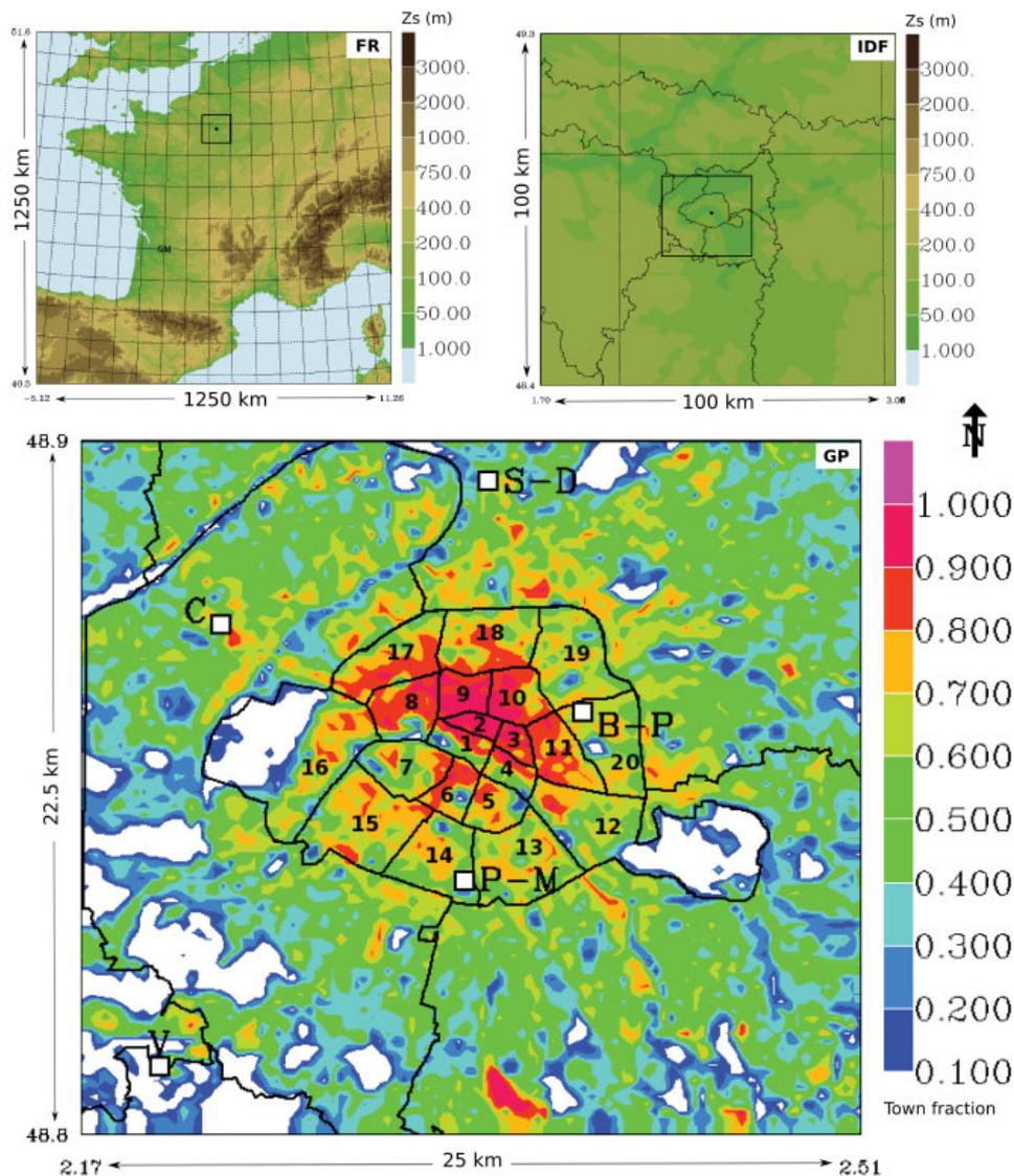
Figure 2. The three-nested simulation domains for the three spatial resolutions (FR: 2.5 km; IDF: 1.25 km; GP: 250 m). Orography ( $Z_s$ ) is shown for FR and IDF, town fraction for GP. On GP domain are also annotated the locations of 5 weather stations (V for Villacoublay, C for Courbevoie, S-D for Saint-Denis, B-P for Belleville-Park, P-M for Paris-Montsouris) and inner Paris district numbers.
