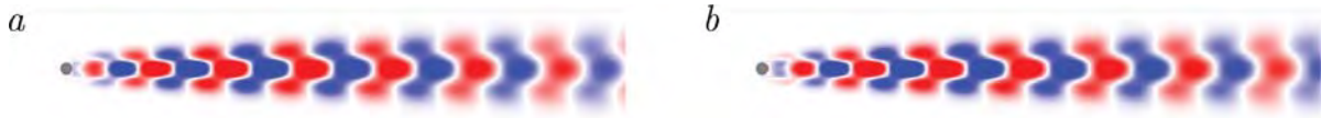
Fig. 2. Spatial distribution of the vorticity for the real (a) and imaginary (b) parts of the unstable eigenmode of the flow past a fixed circular cylinder at Re = 50 .
